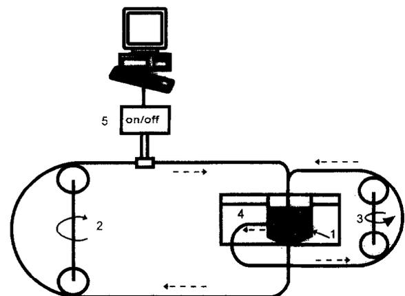
Fig. 9. Scheme of experimental arrangement with the second pump to simulate ultrasound streaming. 1—Container with blood suspension, 2—first pump, 3—second pump, 4—water bath, 5—CW Doppler detection device with computer.
