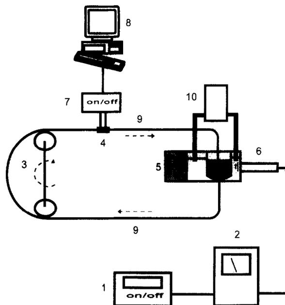
Fig. 1. Scheme of the CW Doppler experimental arrangement. 1—Wave generator, 2—amplifier, 3—pump, 4—measurement chamber, 5—container, 6—ultrasound transducer, 7—CW Doppler device, 8—personal computer, 9—tubes, 10—thermostat.
