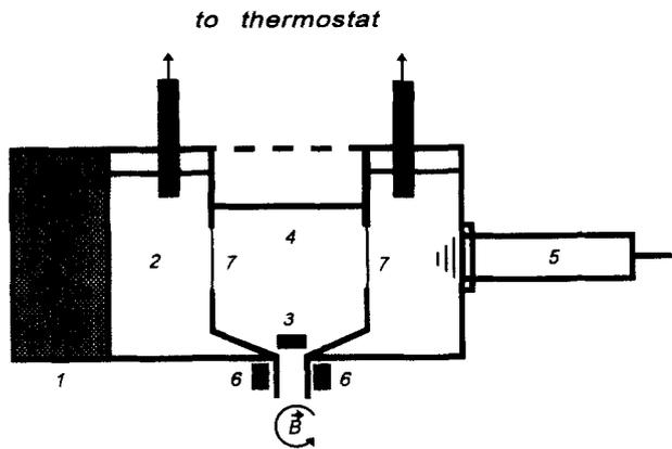
Fig. 2. Scheme of the container for blood samples sonication or stirring. 1—Oil absorber, 2—water bath, 3—magnetic stirrer bar, 4—erythrocyte suspension, 5—transducer, 6—magnetic coils inducing a rotating magnetic field, 7—acoustic windows.
