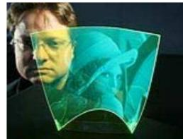
The new imager, which resembles a flexible plastic film, uses fluorescent particles to capture incoming light and channel a portion of it to an array of sensors framing the sheet. With no electronics or internal components, the imager's elegant design makes it ideal for a new breed of imaging technologies, including user interface devices that can
