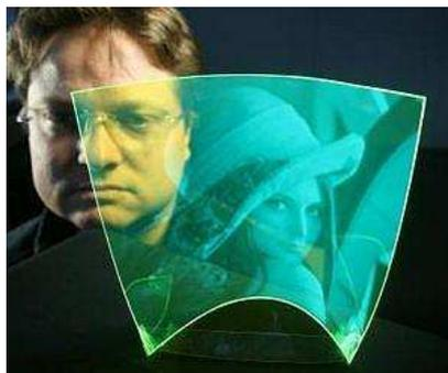
This shows the world's first flexible and completely transparent image sensor. The plastic film is coated with fluorescent particles. Credit: Credit: Optics Express.
