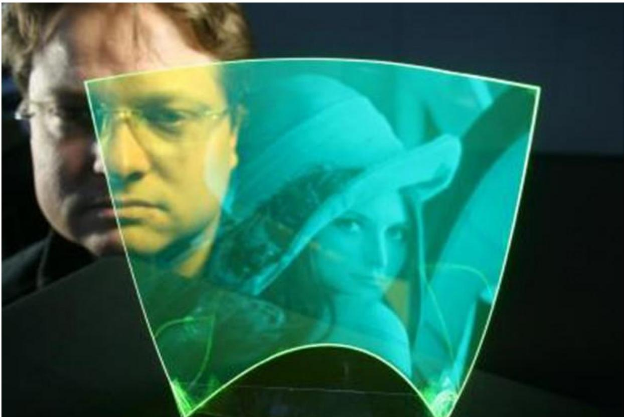
Image Caption: This shows the world's first flexible and completely transparent image sensor. The plastic film is coated with fluorescent particles. Credit: Optics Express.
