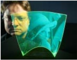
The world's first flexible and completely transparent image sensor. The plastic film is coated with fluorescent particles. Credit: Optics Express.
