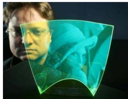
*This shows the world's first flexible and completely transparent image sensor. The plastic film is coated with fluorescent particles. Credit: Optics Express*
