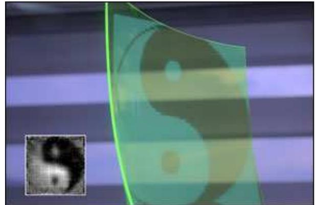
The first prototypes have a low resolution of 32 × 32 pixels because of limited signal-to-noise ratio of the low-cost photodiodes being used. The researchers are planning better prototypes that cool the photodiodes to achieve higher signal-to-noise ratios.
