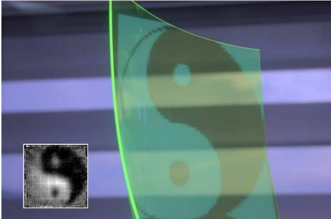
A comparison between the (ground truth) image being focused on the sensor surface and the reconstructed image (inset).
