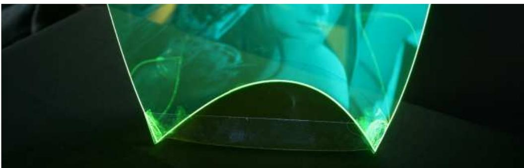
The world's first flexible and completely transparent image sensor. The plastic film is coated with fluorescent particles. Credit: Optics Express.
