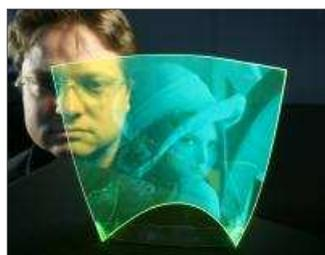
**This shows the world's first flexible and completely transparent image sensor. The plastic film is coated with fluorescent particles.**
