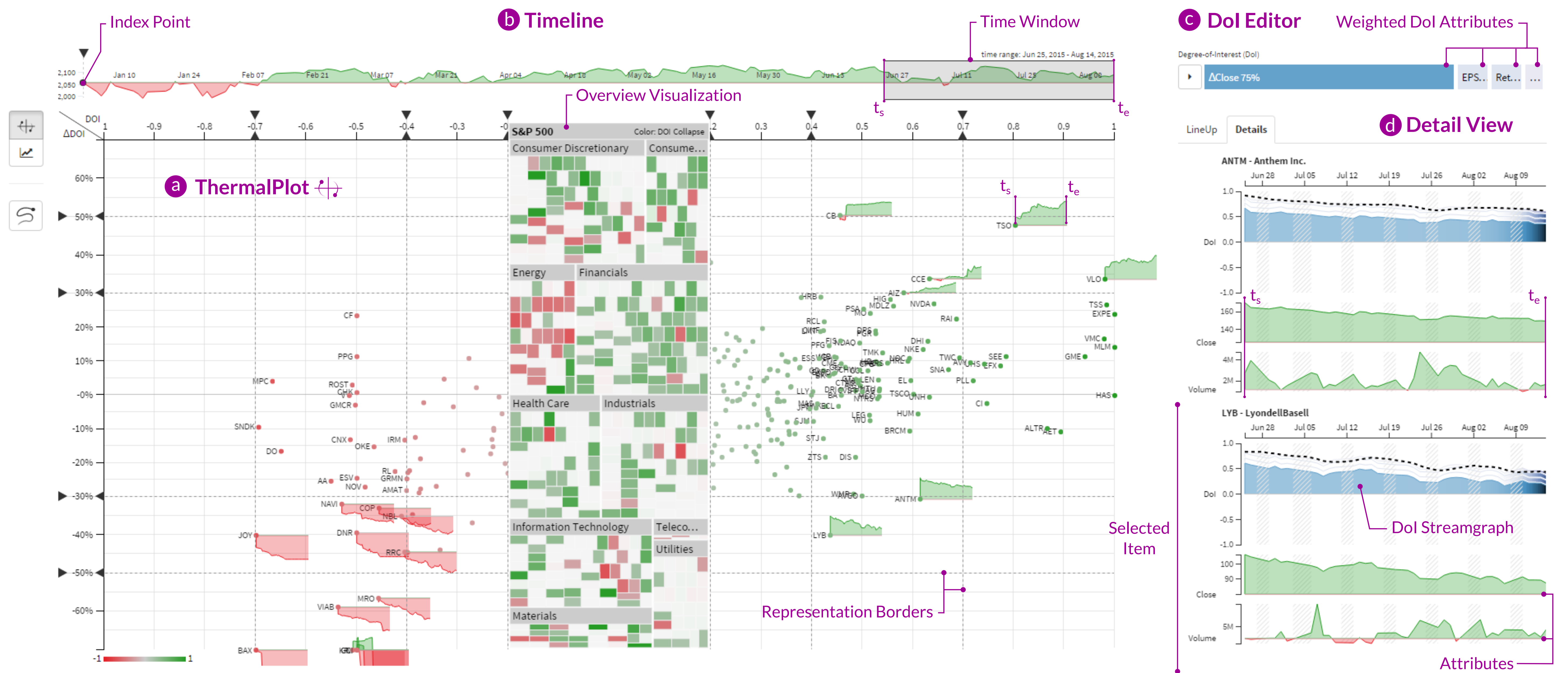
Figure 1: The ThermalPlot technique (a) integrated in the exploration environment for multi-attribute time-series data showing the development of companies listed in the S&P 500 index within a user-specified time window (b). Item positions in the plot are based on the selected index point and the weighted degree-of-interest (DoI) attributes configured with the DoI editor (c). The detail view (d) shows the development of the composed DoI over time as streamgraphs and the line charts of single attributes for selected items.
