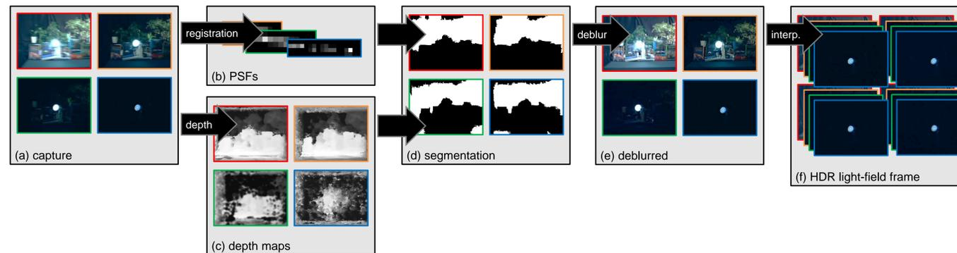
**Figure 2:** An outline of our technique showing four captured perspectives of a camera array (a), local PSFs computed by registration (b), depth maps for each exposure perspective (c), segmentations based on PSFs and depths (d), the deblurred exposure perspectives (e), and the final HDR light-field frame with interpolated exposure perspectives (f).
