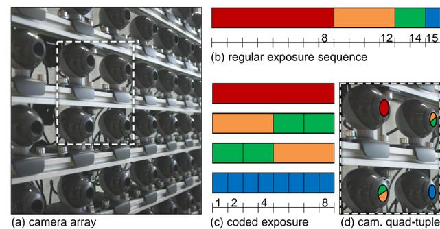
**Figure 1:** Our camera array (a), corresponding recording intervals for capturing a regular exposure sequence (b), our coded exposure approach (c). The exposure pattern is repeated for each camera quad-tuple of the array (d).
