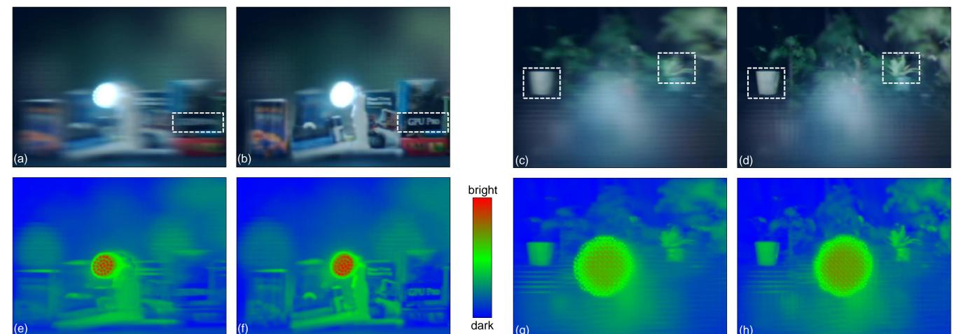
**Figure 4:** Light-field rendering of an HDR light field recorded with regular exposure sequencing (a,c,e,g) and our coded exposure approach (b,d,f,h), where (a,b,c,d) are tone-mapped and (e,f,g,h) are heat-mapped to illustrate the dynamic range of the scene. The synthetic focus of the light-field renderings is set to the foreground (a,b,e,f) and to the background (c,d,g,h).
