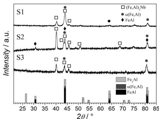
**Figure 3** X-ray diffractograms of the alloys obtained by arc melting showing the presence of an FeAl phase and (Fe,Al)<sub>2</sub>Nb Laves phase, together with the powder diffraction patterns for FeAl, α(Fe,Al) and Fe<sub>3</sub>Al.
