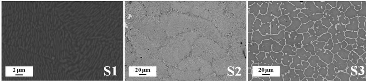
**Figure 1** SEM micrographs of the re-melted samples possessing two present intermetallic phases. A minimum number of primary dendrites of the Laves phase is present in both S1 and S2 as visible in the upper left corner of S2.
