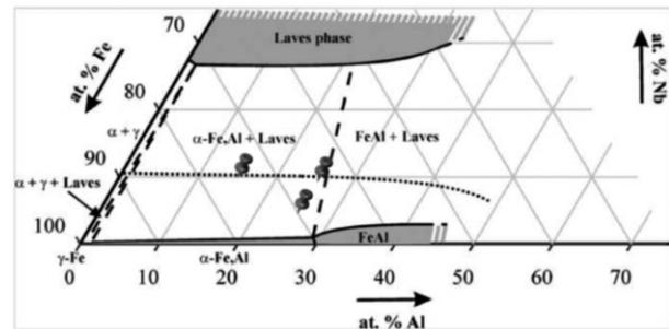
**Figure 2** Partial isothermal cross-section of the FeAlNb system in the Fe-rich corner at 1000 °C [20]. The three pins mark the overall composition of the investigated alloys within the phase diagram.
