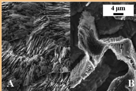
SEM micrograph of (A) Fe-15Al-10Nb and (B) Fe-26Al-4Nb after anodisation in 0.4 M borate buffer.
