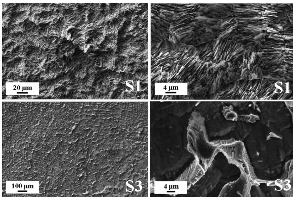
**Figure 4** SEM micrographs showing the morphology after anodisation in 0.4 M borate buffer. The upper micrographs show aligned lamellar to fibrous structures of the light grey  $(\text{Fe,Al})_2\text{Nb}$  phase of sample S1. The lower micrographs depict the obtained branched structures protruding from the dissolved  $\alpha(\text{Fe,Al})$  phase of sample S3.
