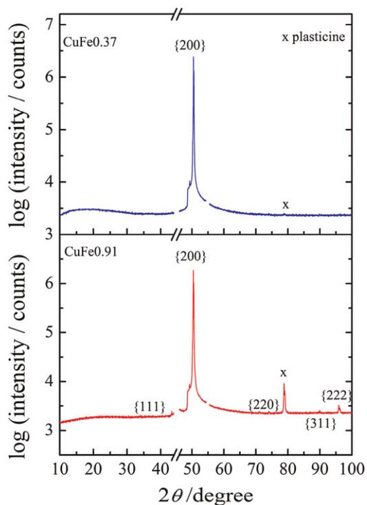
**Figure 3** (online colour at: [www.pss-a.com](http://www.pss-a.com))  $2\theta$  XRD scans of CuFe<sub>0.37</sub> (top) and CuFe<sub>0.91</sub> (bottom). Since the {200}  $K_{\beta}$  peak at  $2\theta \sim 45^{\circ}$  showed no important information, this region was cut out.
