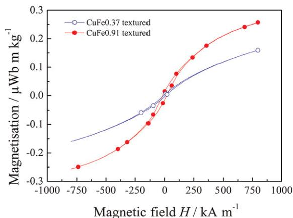
**Figure 6** (online colour at: [www.pss-a.com](http://www.pss-a.com)) Magnetisation loops of CuFe0.37 and CuFe0.91 at 5 K.
