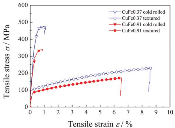
**Figure 7** (online colour at: [www.pss-a.com](http://www.pss-a.com)) Stress–strain curves for the rolled and textured Cu–Fe alloys.
