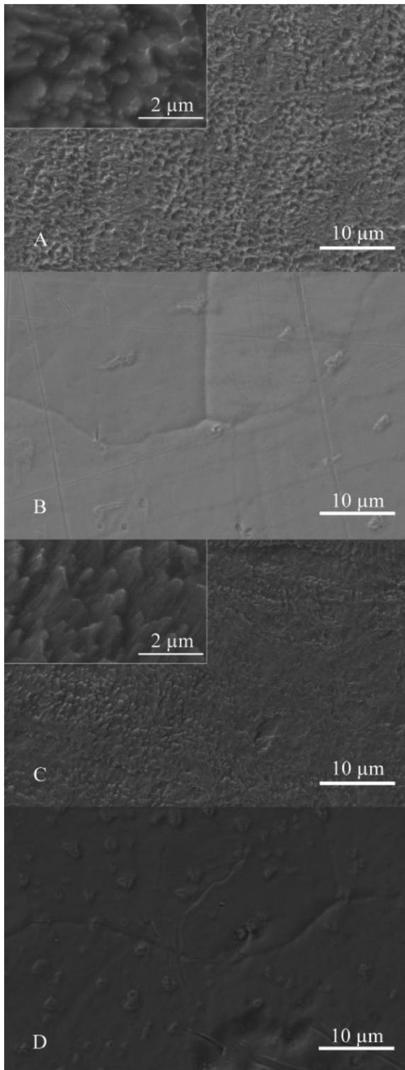
**Figure 1** SEM micrographs of CuFe<sub>0.37</sub> (A and B) and CuFe<sub>0.91</sub> (C and D) showing the microstructure of the cold rolled (A and C) and heat treated (B and D) specimen.
