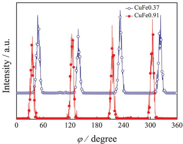
**Figure 4** (online colour at: [www.pss-a.com](http://www.pss-a.com)) Phi scans of CuFe0.37 and CuFe0.91, giving FWHM values of 7.3 and 6.8°, respectively.
