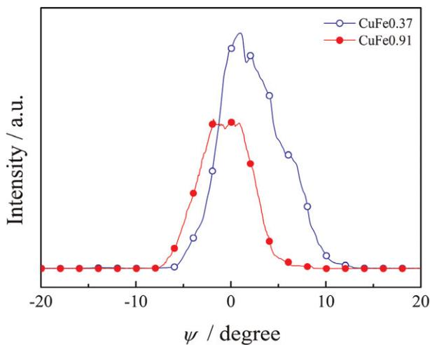
**Figure 5** (online colour at: [www.pss-a.com](http://www.pss-a.com)) Psi scans of CuFe0.37 and CuFe0.91. Similar FWHM values of 7.2° are retrieved for both alloys.
