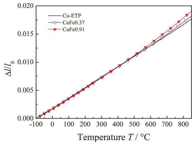
**Figure 2** (online colour at: [www.pss-a.com](http://www.pss-a.com)) Comparison of the thermal expansion.
