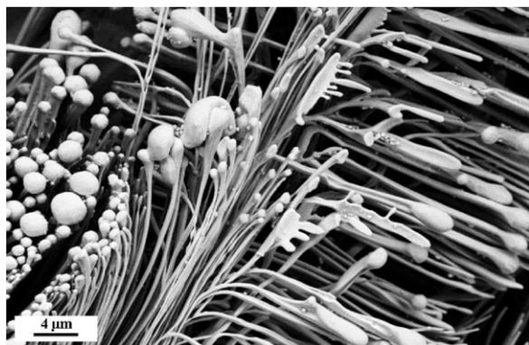
**Figure 6** WCr (50:50) alloy nanowires partially showing growth irregularities and branched structures.
