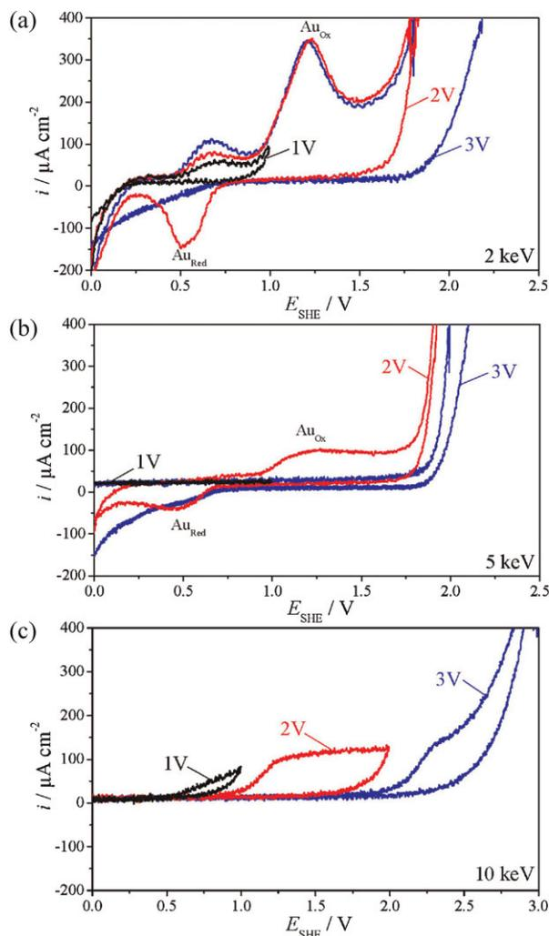
**Figure 4** (online colour at: [www.pss-a.com](http://www.pss-a.com)) Cyclic voltammograms recorded during repassivation of Au implanted anodic  $\text{Al}_2\text{O}_3$ .
