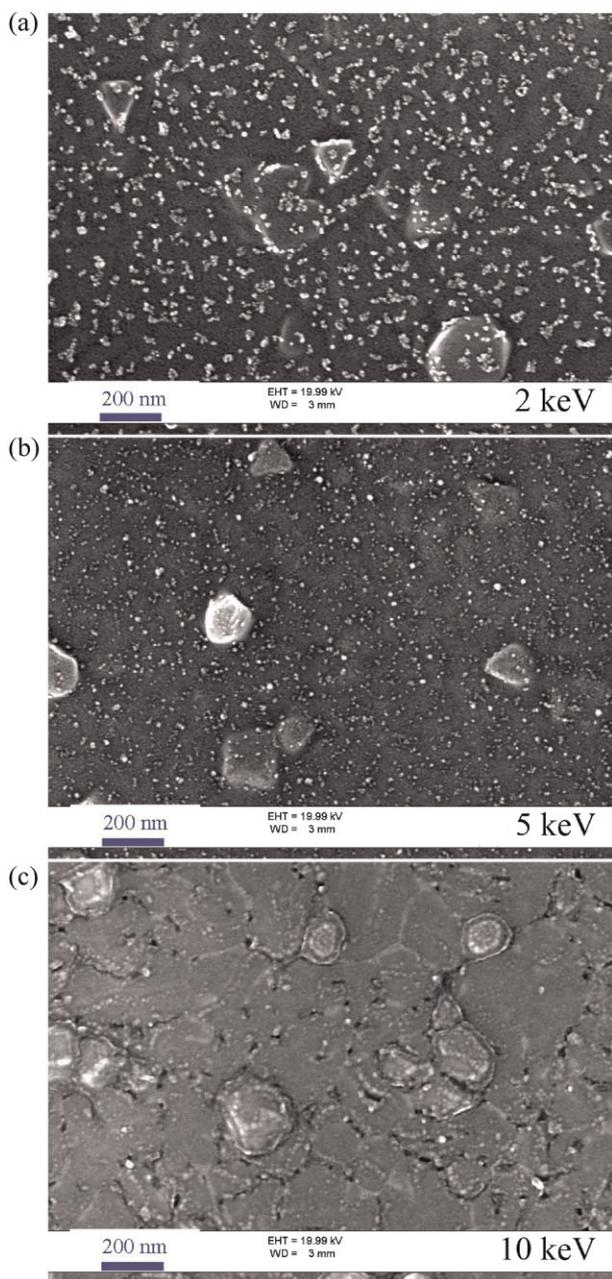
**Figure 2** (online colour at: [www.pss-a.com](http://www.pss-a.com)) SEM images of Al<sub>2</sub>O<sub>3</sub> surfaces immediately after Au implantation at different (a) 2, (b) 5 and (c) 10 keV energies.
