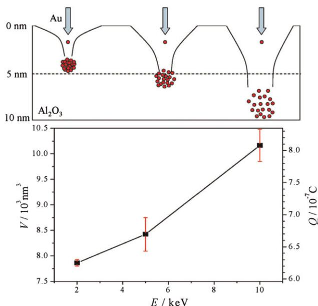
**Figure 5** (online colour at: [www.pss-a.com](http://www.pss-a.com)) Schematic drawing of the implantation process in alumina and the calculated sputtered volumes versus the ion impact energy.
