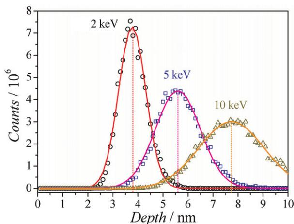
**Figure 1** (online colour at: [www.pss-a.com](http://www.pss-a.com)) SRIM calculation of the stopping range of Au ions implanted in  $\text{Al}_2\text{O}_3$  with different energies.
