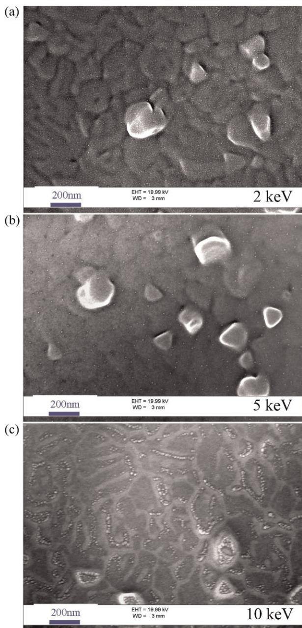
**Figure 3** (online colour at: [www.pss-a.com](http://www.pss-a.com)) SEM images of  $\text{Al}_2\text{O}_3$  surfaces immediately after electrochemical repassivation.
