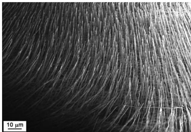
**Figure 1** SEM image of tungsten nanowire array. Partially exposed wires protrude from the NiAl matrix. The nanowires' diameter is 200 nm, exposed length is 20  $\mu\text{m}$ .
