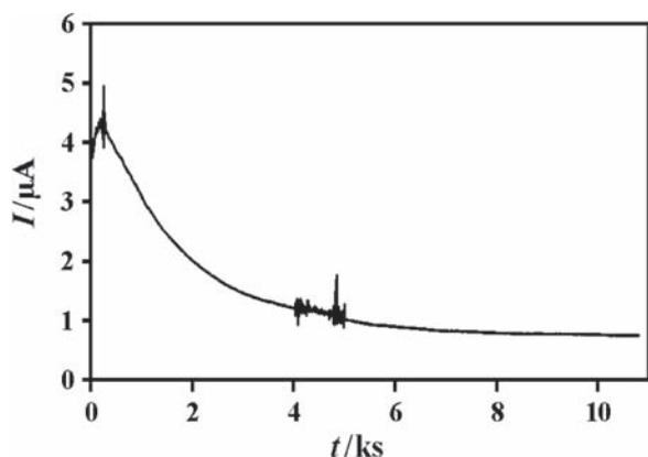
**Fig. 9.** Current transient of the selective electro-dissolution of the Mo nanowires in an acetate buffer (pH 6.0) at 0.2 V (SHE).
