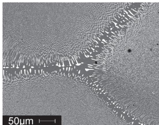
**Fig. 1.** Cellular eutectic structure of the *ds*-NiAl–Mo alloy grown at 30 mm h<sup>-1</sup>. The sample was cut in a direction perpendicular to the growth direction and subsequently polished.
