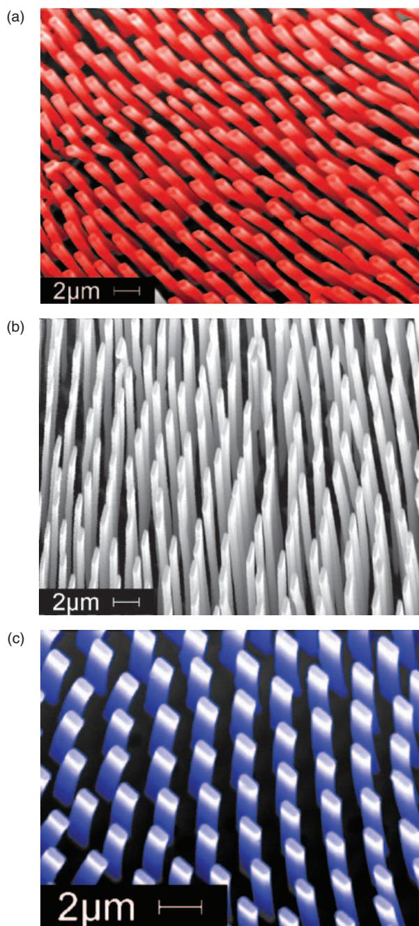
**Fig. 6.** Array of the Mo nanowires partially released from the NiAl matrix at different magnifications.
