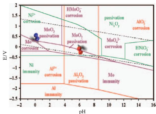
Fig. 4. Combined simplified pH-potential stability diagram derived from Pourbaix diagrams of the three elements Ni, Al and Mo.
