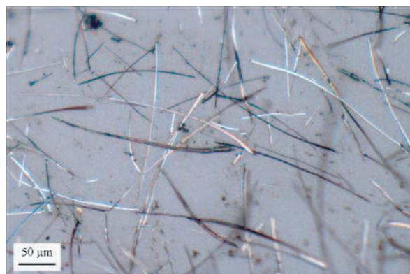
**Fig. 7.** Mo nanowires on a filter paper after complete dissolution of the matrix.
