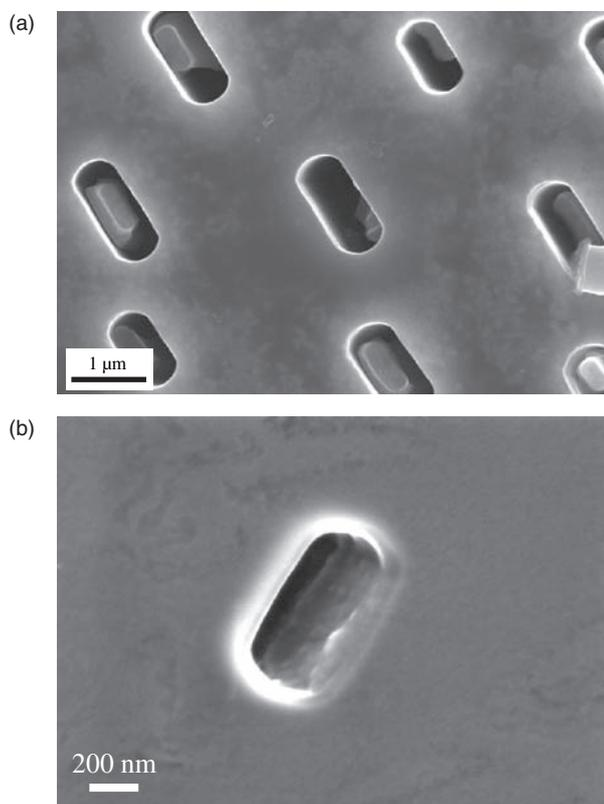
**Fig. 8.** (a) Nanopore array in a *ds*-NiAl-Mo eutectic alloy after selective electrodisolution of the Mo-minor phase in an acetate buffer (pH 6.0) at  $0.2 \text{ V (SHE)}$ . (b) Close view of a single nanopore.
