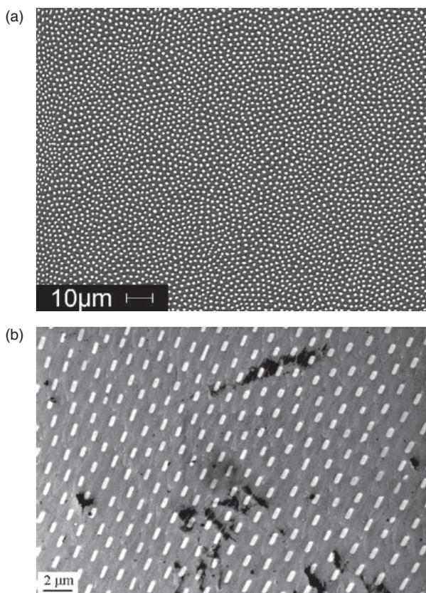
**Fig. 2.** Morphology of the Mo fibers embedded in the NiAl matrix at different magnifications. See Figure 1 for experimental details.
