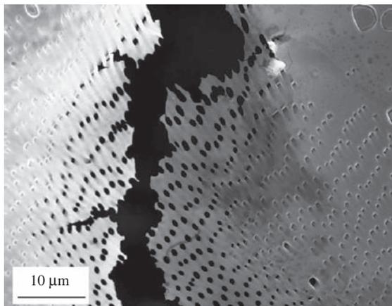
**Fig. 10.** Nanofilter generation through complete wire dissolution.
