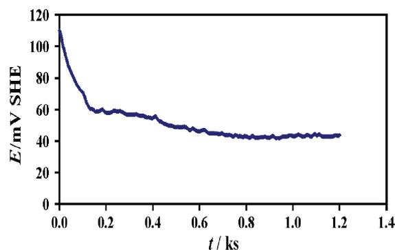
Fig. 5. Potential transient of matrix dissolution of *ds*-NiAl-Mo in a mixture of 3.2% HCl and 3% H<sub>2</sub>O<sub>2</sub>.
