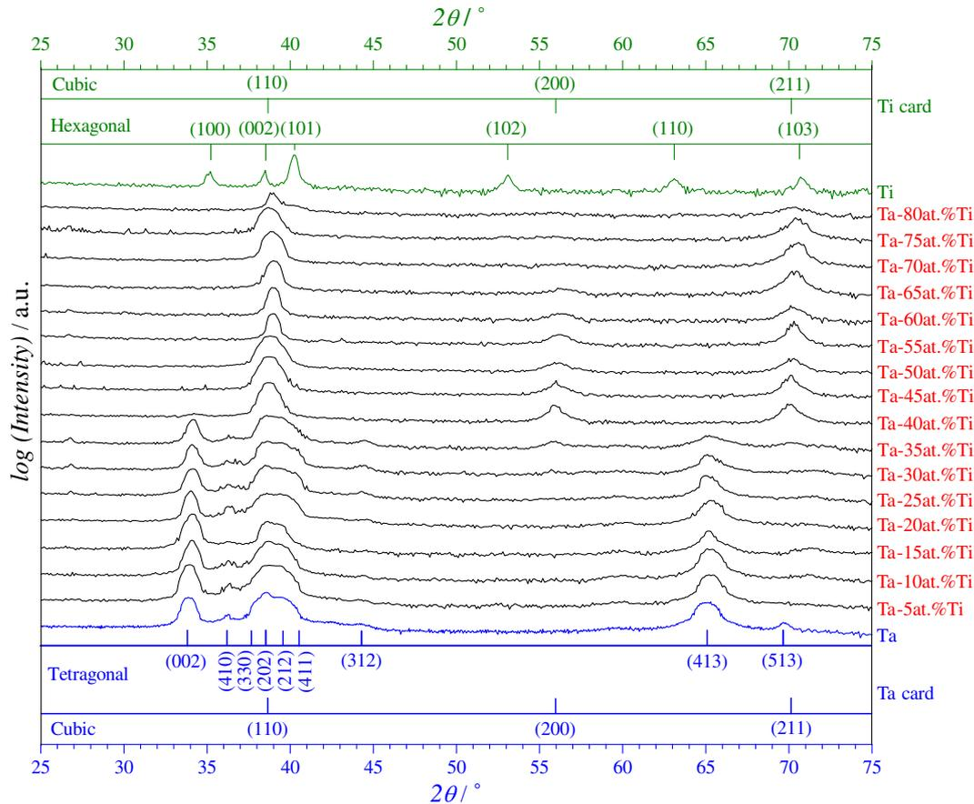
Fig. 2. XRD patterns measured locally for different concentrations on the Ta–Ti composition spread.
