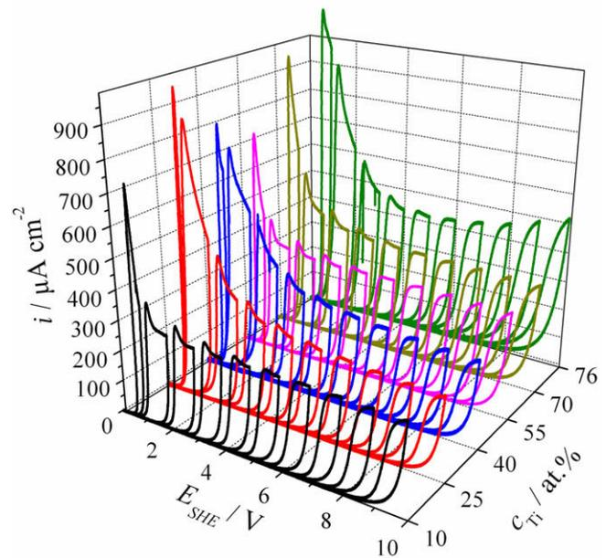
Fig. 3. Cyclic voltammograms recorded during the potentiodynamic oxide growth on Ta–Ti binary alloys for different concentrations.
