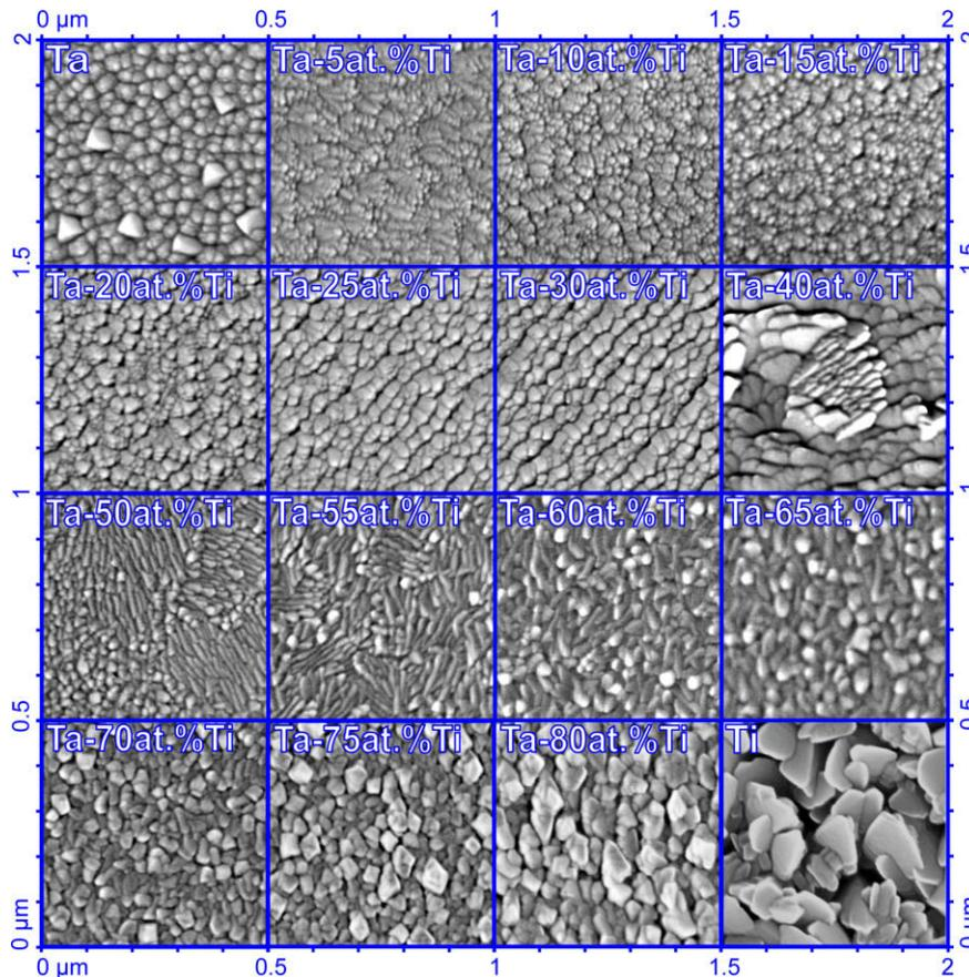
Fig. 1. SEM images of the surface of the Ta–Ti binary composition spread for different concentrations. The surfaces of pure Ti and Ta are presented as references.
