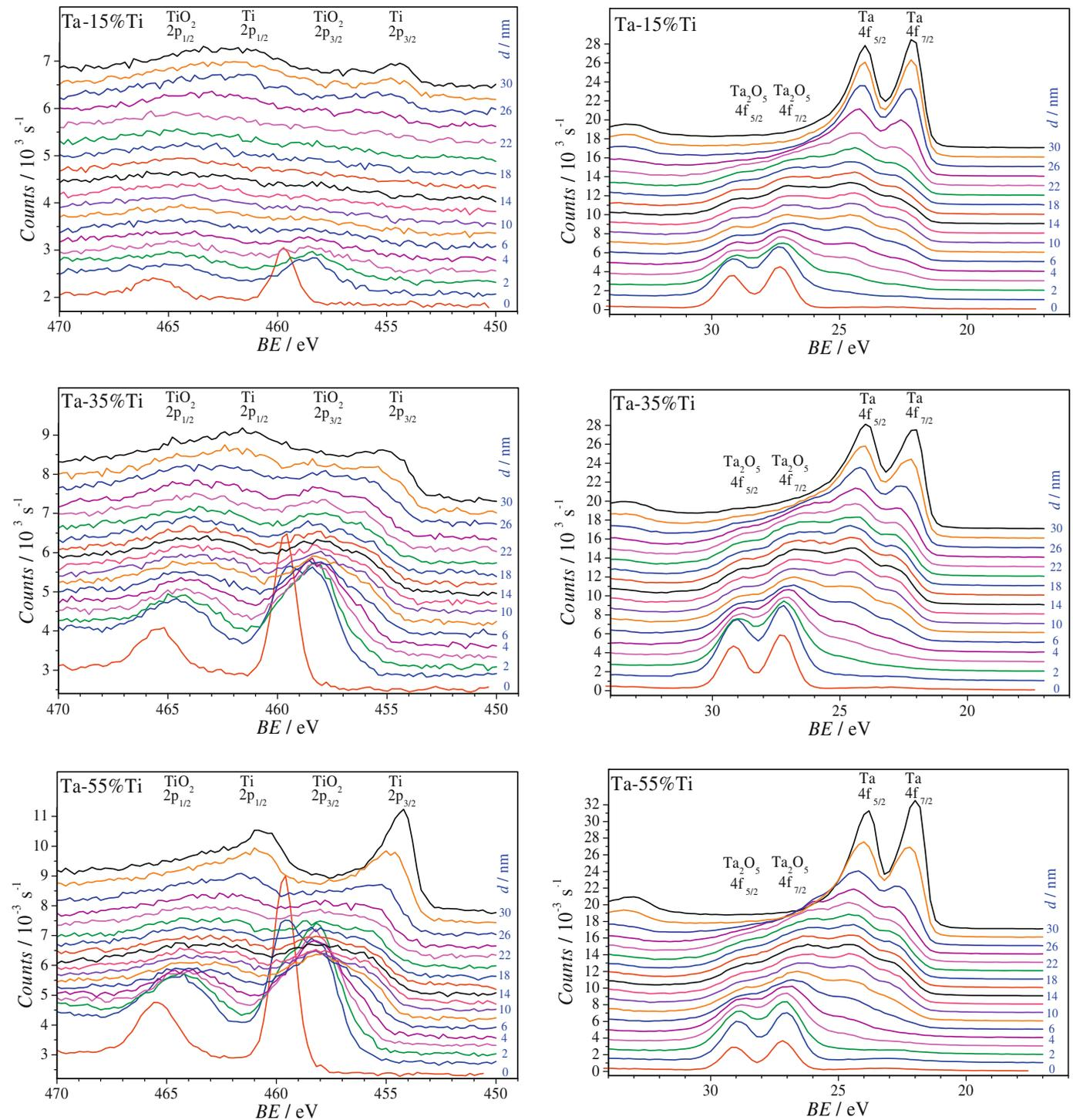
Fig. 7. XPS depth profiling spectra of the anodic oxides potentiodynamically grown at 10 V on the Ta-Ti composition spread at different compositions.
