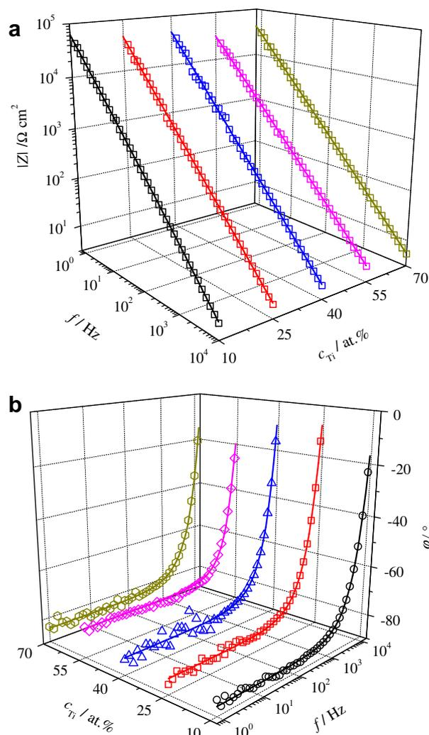
Fig. 4. Electrochemical impedance spectroscopy measurements of the anodic oxides grown potentiostatically at 3 V on the Ta–Ti composition spread for different concentrations.
