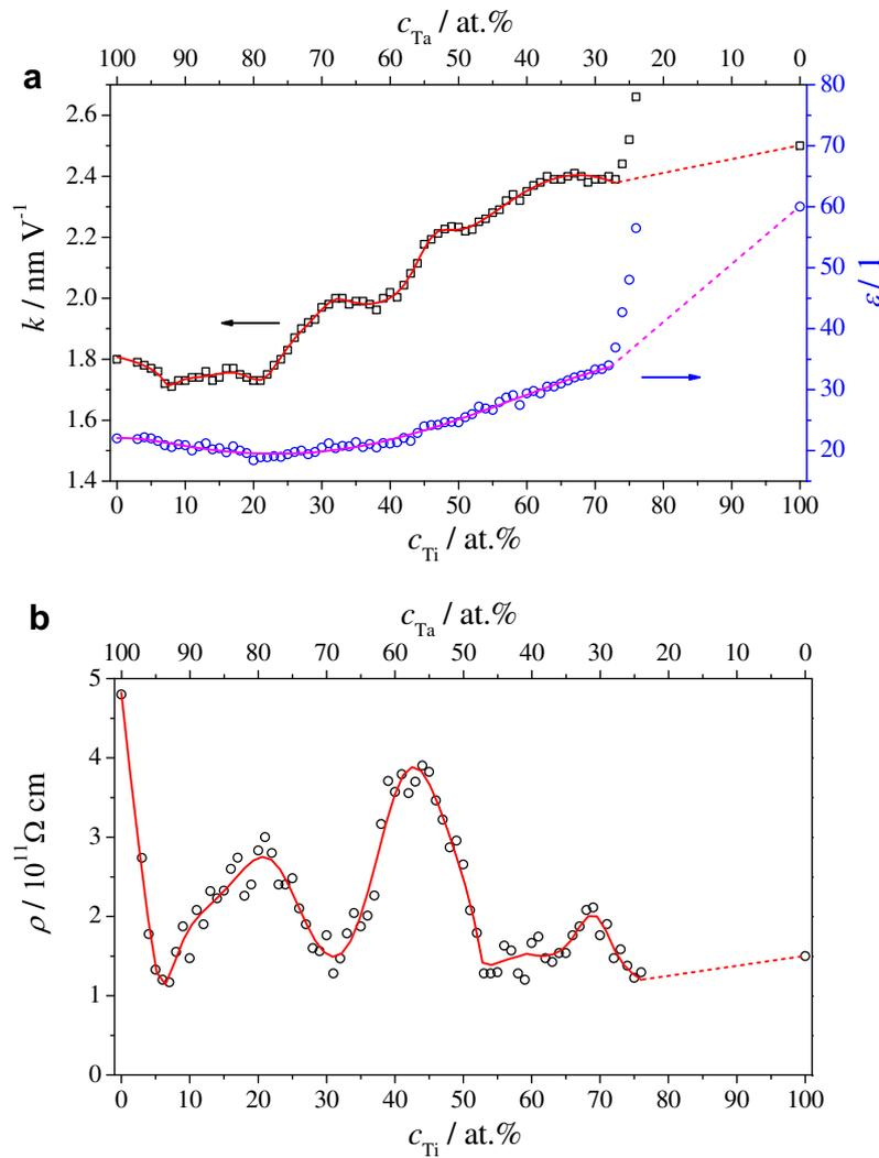
Fig. 5. (a) Oxide formation factors, dielectric constants and (b) electrical resistivities for the anodic oxides grown on the Ta–Ti binary composition spread.
