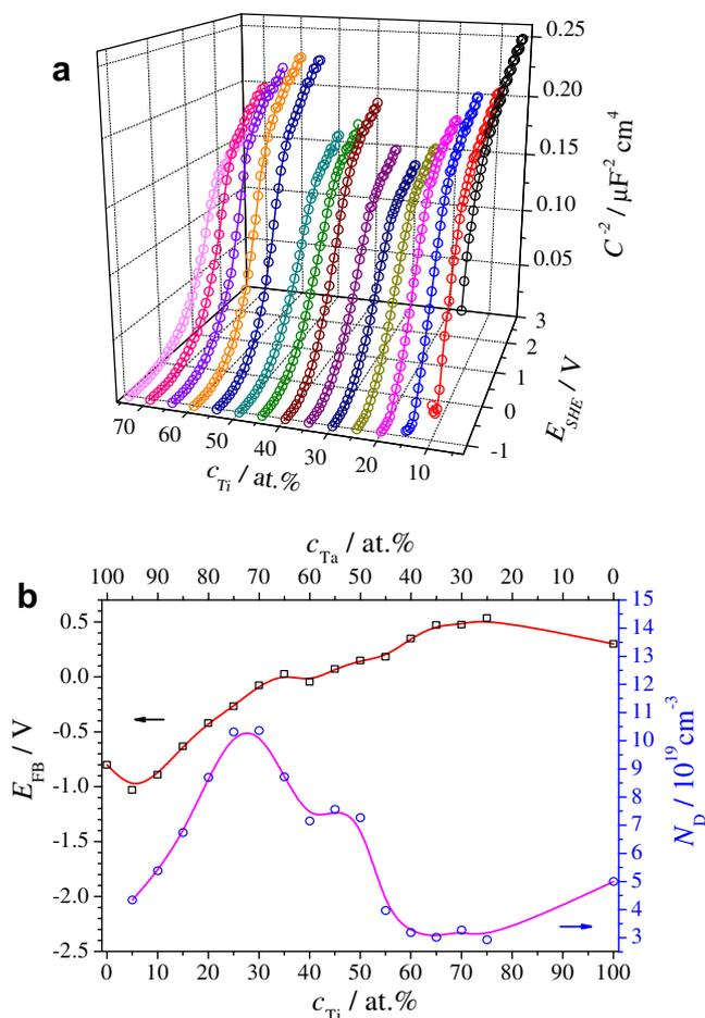
**Fig. 6.** (a) Mott–Schottky plots and (b) flat band potentials and donor densities for the anodic oxides grown on the Ta–Ti composition spread at different concentrations.
