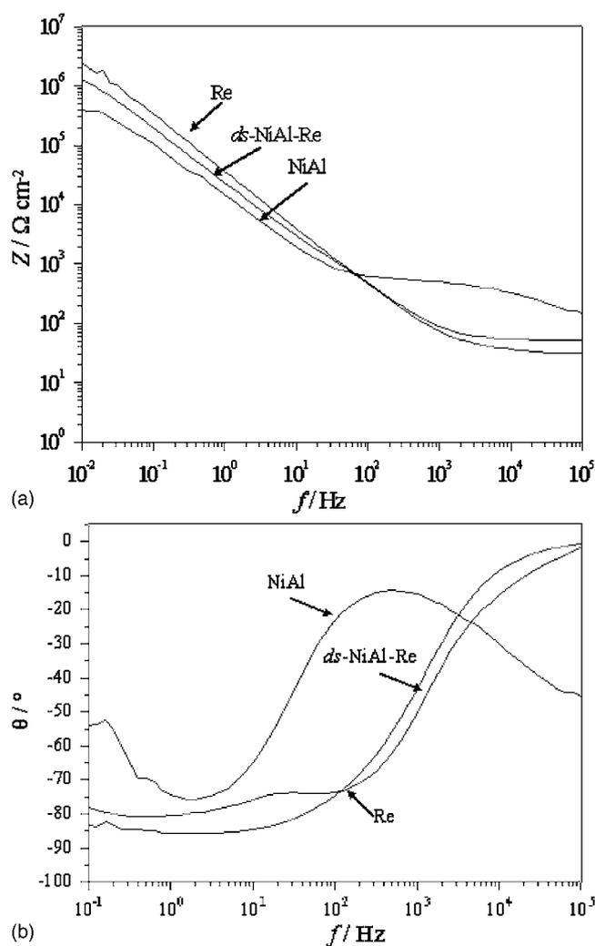
**Figure 6.** Frequency dependence of  $Z$  and phase-angle  $\theta$  for NiAl-Re (light gray line), NiAl (black line), and Re (gray line) after polarization in acetate buffer (pH 6.0) at 0.7 V vs SHE.
