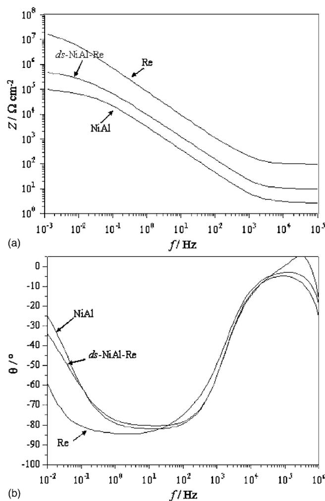
**Figure 3.** EIS spectra obtained for NiAl, Re, and NiAl-Re after polarization of the samples in acetate buffer for passivation of the matrix at 0 V.
