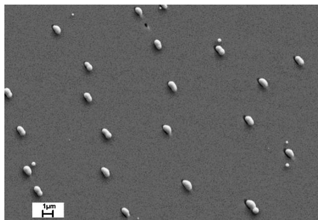
**Figure 11.** Au deposits observed on a ds-NiAl-Re sample after pretreatment at 0.7 V.
