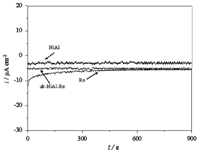
Figure 2. Current transients recorded for the polarization of NiAl, Re, and ds-NiAl-Re in neutral acetate buffer (pH 6.0) at 0 V (vs SHE).
