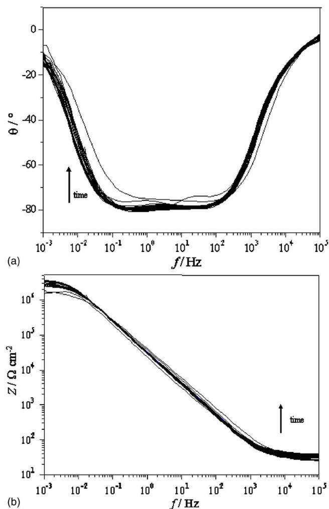
**Figure 7.** Frequency dependence of  $Z$  and phase-angle  $\theta$  for NiAl-Re after polarization in acetate buffer (pH 6.0) at 0.7 V vs SHE for increasing times.
