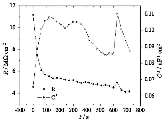
**Figure 8.** Evolution of resistance and inverse of capacitance for NiAl-Re after longer polarization times at 0.7 V.
