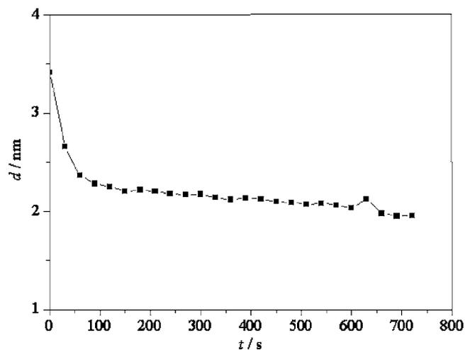
**Figure 9.** Decrease in thickness of the  $\text{Al}_2\text{O}_3$  and NiO oxide layer for the NiAl-Re system after longer polarization times at 0.7 V.
