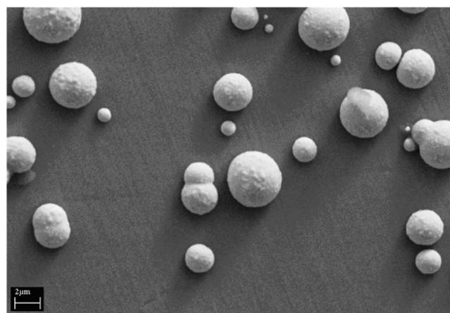
**Figure 4.** Gold deposited on a NiAl-Re sample after polarization at 0 V.
