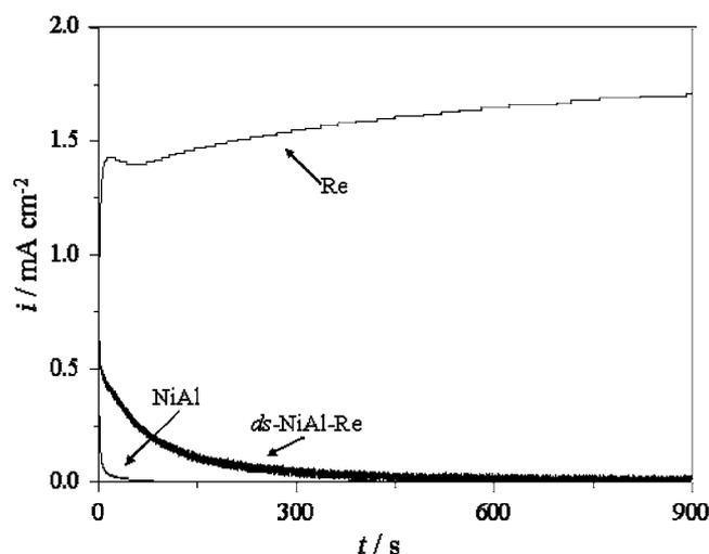
**Figure 5.** Current transients recorded after polarization of NiAl, NiAl-Re, and Re samples at 0.7 V in acetate buffer pH 6.0.
