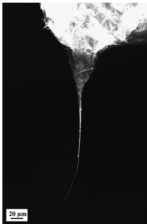
Fig. 1. SEM picture of the tungsten nano wire protruding from the NiAl matrix.
