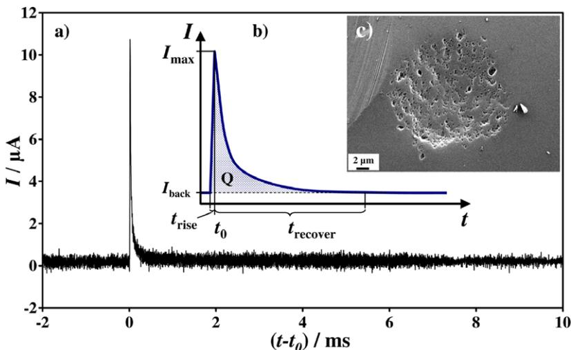
Fig. 4. (a) Current transient normalised to the time of peak current  $t_0$ . (b) Schematic current transient with all characteristic parts marked. (c) SEM-micrograph of the resulting crater.
