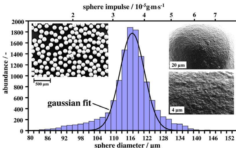
Fig. 3. Distribution of abrasive particle sizes. The upper x-axis shows the sphere impulse calculated for a speed of  $7 \text{ m s}^{-1}$ . The most abundant diameter is  $117 \mu\text{m}$ . The insets show SEM-micrographs of the abrasive particles at different magnifications.
