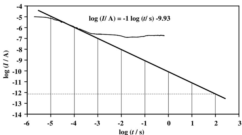
Fig. 5. Double logarithmic plot of the data from Fig. 4a. The equation describes the fit applied to the high field part of the plot. The intercept of this fit with the time value of 100 s yields an approximation of the repassivation current.
