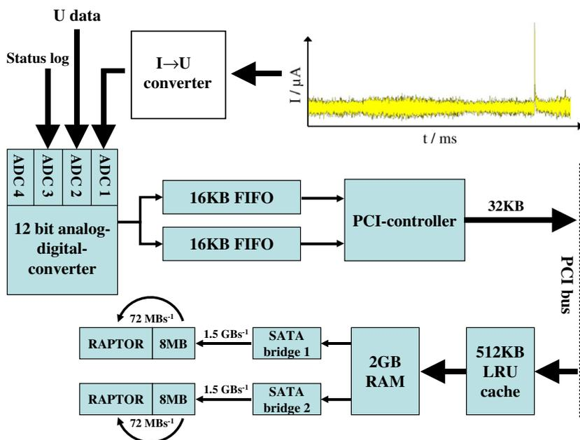
Fig. 2. Simplified chart of the high speed data acquisition and storage system used. Detailed description is given in the text.
