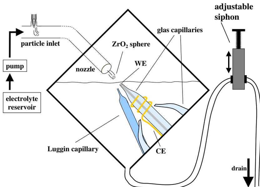
Fig. 1. Schematic of the Slurry jet impingement system. The slurry ejecting nozzle faces the immersed working electrode (WE) and can be adjusted by a  $xy$ -stage. Counter and reference electrode are in close vicinity of the WE. The adjustable siphon allows precise control of the electrolyte level in the chamber.
