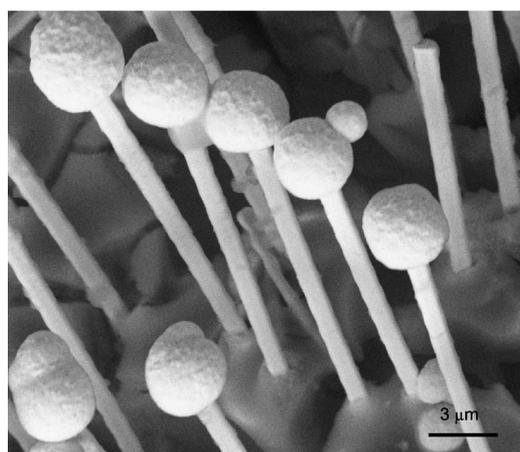
**Figure 4.** SEM image of gold microspheres deposited onto rhenium nanofibers after chemical etching of the NiAl matrix.
