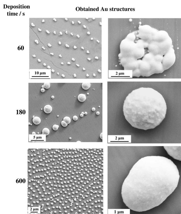
**Figure 3.** SEM images of gold deposits obtained on passive NiAl-Re samples after different polarization times.
