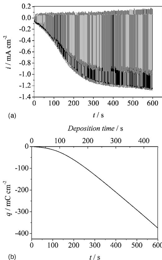
**Figure 2.** (a) Current density recorded over polarization time for the application of cathodic and anodic pulses (ratio 3:1 s) on a passivated NiAl–NRe eutectic (working electrode). A gold foil was employed as counter electrode. (b) Charge obtained after integration of the recorded  $i$  vs  $t$  plot (same conditions as expressed for Fig. 2a).
