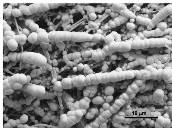
**Figure 5.** SEM image of gold deposits obtained when the NiAl-Re samples are not preconditioned for passivation of the NiAl matrix.
