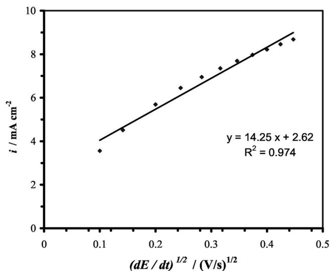
**Figure 7.** Increase in the anodic peak current with scan rate for 0.1 M ferrocyanide as recorded with the array of deposited gold structures as working electrode. A commercial Ag/AgCl electrode was employed as reference, and a gold foil as counter electrode.
