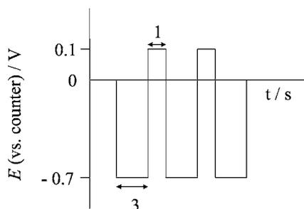
**Figure 1.** Schematic representation of the reverse polarization pulses applied for gold electrodeposition.
