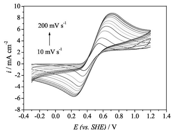
**Figure 6.** Cyclic voltammograms recorded for 0.1 M ferrocyanide at different scan rates. The gold microspheres deposited onto the rhenium fibers (after 5 min polarization) were employed as working electrode. An Ag/AgCl electrode was used as reference and a gold foil as counter electrode.
