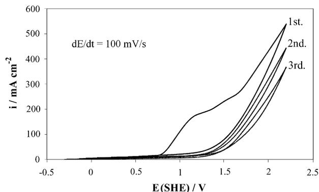
Fig. 5. Cyclic voltammograms consecutively recorded for polished NiAl–Re electrodes in  $0.1$  M acetate buffer pH 6.0 (scan rate =  $100$  mV s<sup>-1</sup>).
