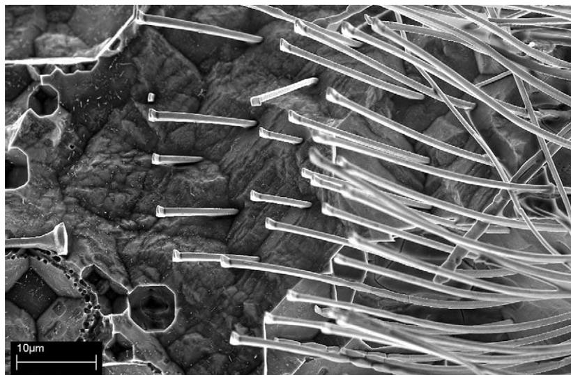
Fig. 4. Re fibers observed in the corroded NiAl matrix after chemical dissolution of the matrix. The aspect ratio, the homogeneous diameter and the parallel assignment are clearly visible.
