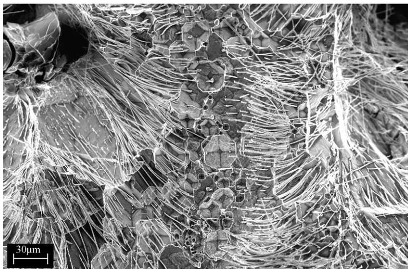
Fig. 3. SEM images of NiAl–Re alloy after digestion in HCl/H<sub>2</sub>O<sub>2</sub>.
