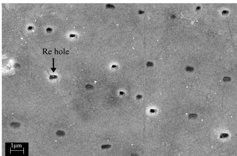
Fig. 7. SEM image of the NiAl–Re alloy after passivation at pH 6.0. The holes present in the structure are attributed to rhenium dissolution to perrhenate.
