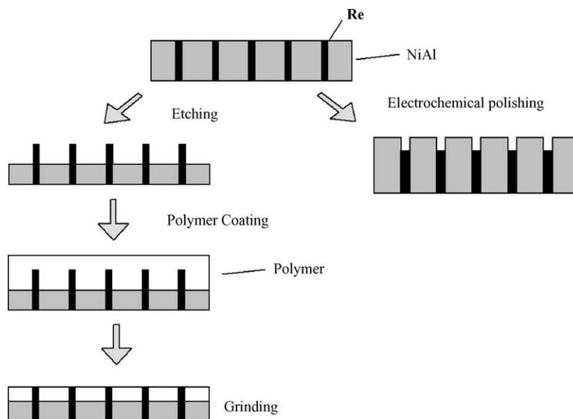
Fig. 2. Schematic of the preparation routes for nanowire arrays and nanopore arrays.
