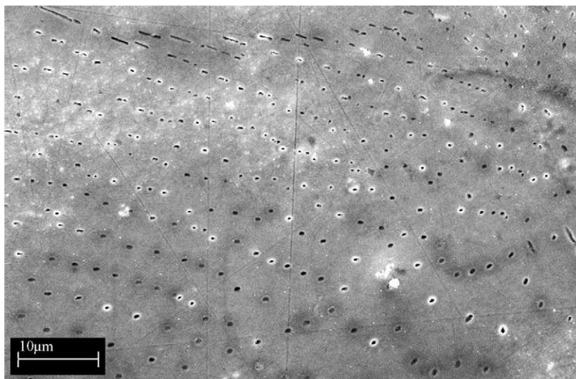
Fig. 6. SEM image of NiAl–Re alloy after electrochemical oxidation at pH 6.0.
