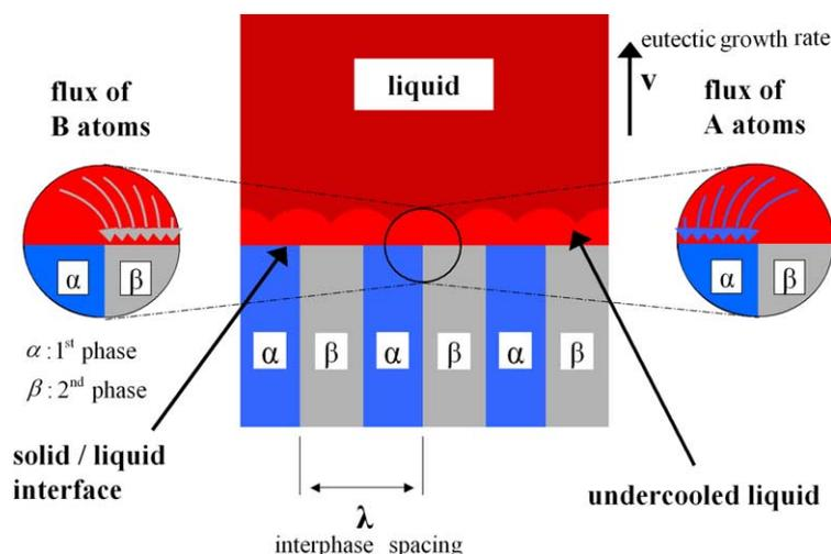
Fig. 1. Schematic of eutectic growth mechanism.
