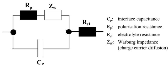
Fig. 4. Equivalent circuit used for fitting the data from the impedance measurements. It is based on the model of a precipitate layer on top of the zinc surface allowing electron and ion transfer as the charge carrier transport mechanism.
