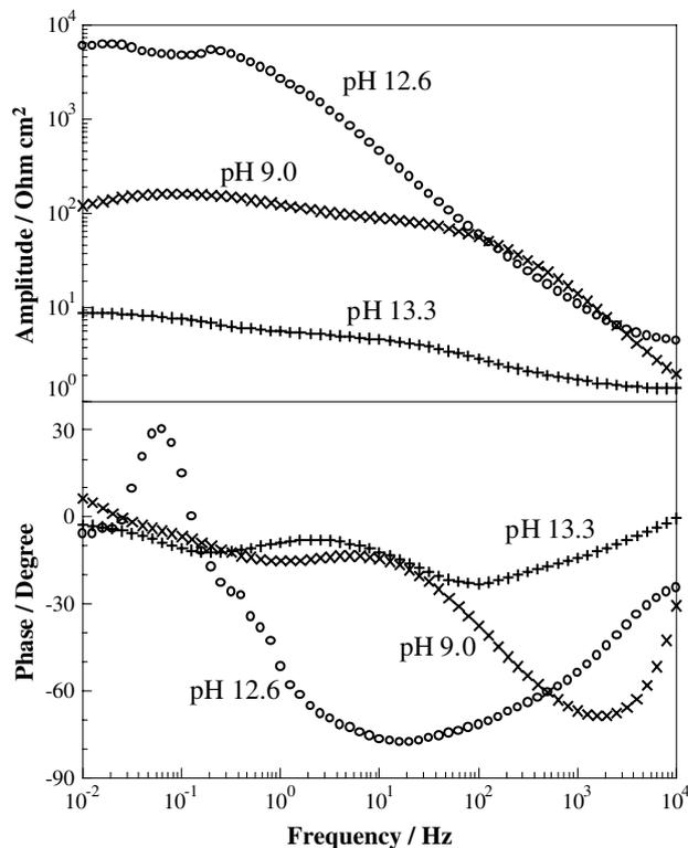
Fig. 3. Measured impedance spectra on zinc in aerated 0.1 M Na<sub>2</sub>SO<sub>4</sub> solution for different pH values adjusted with NaOH. The spectra assigned to the potential maximum at pH = 12.6 shows a significant higher impedance amplitude  $|Z|$  for low frequencies as in case of the other two shown spectra for pH = 9.0 and pH = 13.3. Coupled to this rise is also a greater instability in the measured phase of the taken spectra for the low frequencies.
