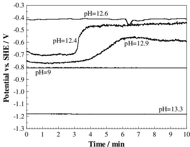
Fig. 1. Measured potential transients on zinc in aerated 0.1 M  $\text{Na}_2\text{SO}_4$  solution for different pH values adjusted with NaOH. The transients for pH = 12.4 and 12.9, assigned to the increase, respectively, decrease to a potential maximum at pH = 12.6 (see Fig. 2), show a significant delay in the potential stabilisation.
