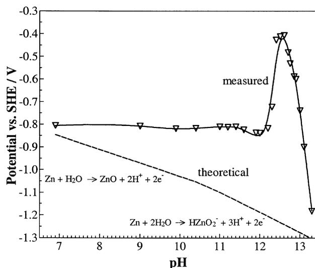
Fig. 2. Corrosion potentials of zinc in aerated 0.1 M  $\text{Na}_2\text{SO}_4$  at different pH values adjusted with NaOH. The potential values were estimated from the potential transients for the particular pH after the potential has been stabilized (see Fig. 1). The theoretical line is calculated based on thermodynamic aspects and hydroxylation at the interface.
