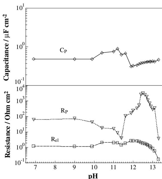
Fig. 5. Values for the interface capacitance and the polarisation resistance of the surface and the forming layer gained from performed impedance spectroscopic measurements on zinc in aerated 0.1 M  $\text{Na}_2\text{SO}_4$  at different pH values adjusted with NaOH.
