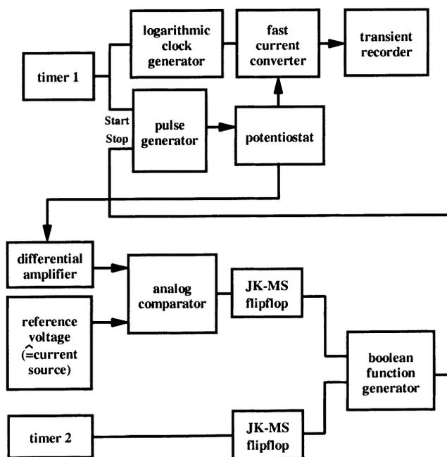
Fig. 2. Schematic diagram of the electronic setup used. Connections with arrows indicate analogue signal flows, line connections indicate digital connections (TTL level). Details are described in the text.
