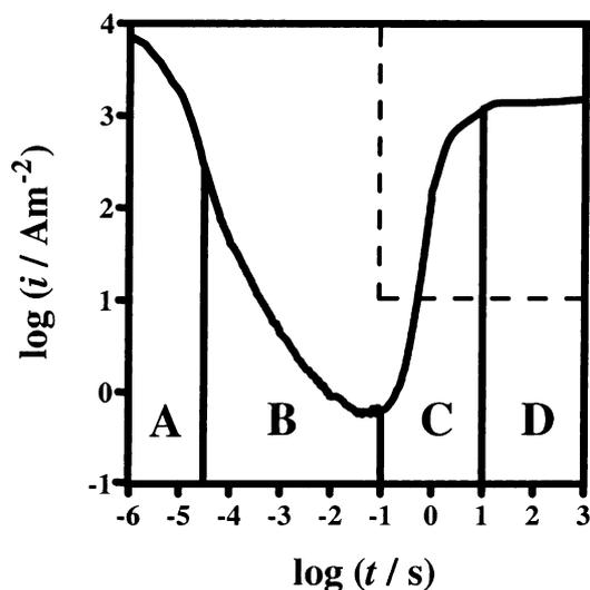
Fig. 1. Current transient of a potentiostatic breakdown of  $\text{Al}_2\text{O}_3$  film ( $d = 4.5$  nm) on Al after a potential jump to  $E_{\text{HESS}} = -2$  V (hydrogen electrode same solution), 25 °C, acetate buffer pH 6.0: (A) charging of the oxide capacity; (B) dielectric relaxation = metastable area; (C) cathodic breakdown of the oxide film; (D) stationary hydrogen evolution. The dashed rectangle in the upper right part indicates prohibited experimental conditions.
