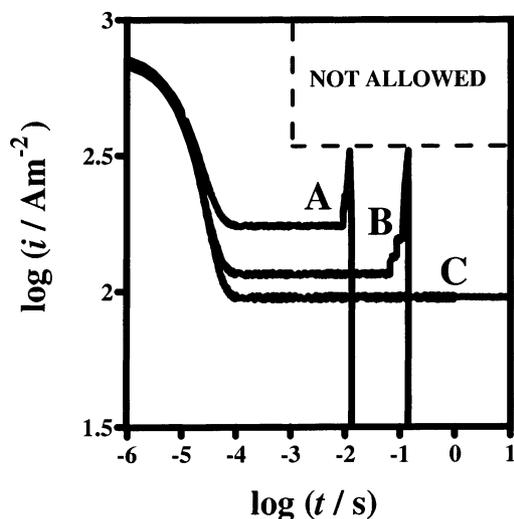
Fig. 3. Subsequent current transients of voltage steps to 3.5 V on a MIM contact (30 nm Al/4.5 nm  $\text{Al}_2\text{O}_3$ /20 nm Ag) using the described switching system: (A) highest tunnel current and shortest time to breakdown; (B) partially annealed sample with lower tunnel current and longer time to breakdown; (C) completely annealed sample with lowest tunnel current and increased breakdown stability.
