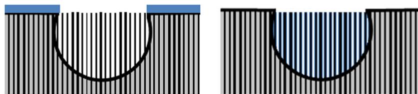
**Fig. 8** Schematic drawings of functionalized microvials coated with a hydrophobic layer the sample surface (*left*) and sputtered with PTFE
