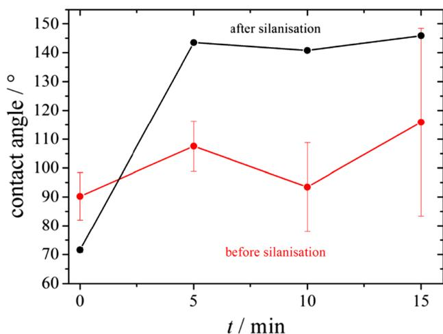
**Fig. 7** Measured contact angles before and after surface functionalisation using OTS as a function of the etching time. Silanisation leads to increased contact angle of etched samples and minimizes the measured error
