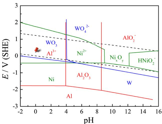
**Fig. 1** Superposition of the Pourbaix diagrams of Ni, Al and W considering lines for an initial concentration of the dissolved species of  $10^{-6}$  M. The red pin indicates the conditions for a simultaneous dissolution of the matrix elements Ni and Al under concurrent oxidation of W
