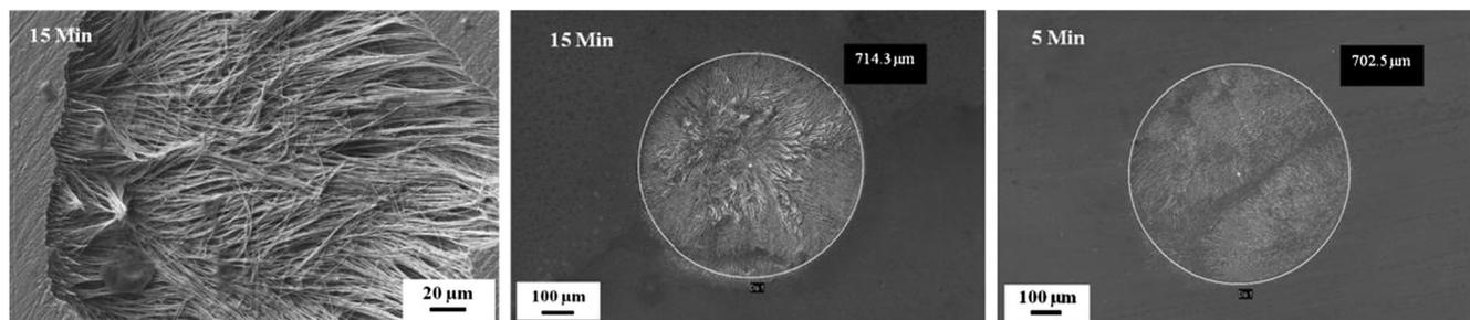
**Fig. 4** Microvials with W-nanowire arrays after selective matrix dissolution of samples cut parallel to the growth direction (left) and perpendicular to the growth direction
