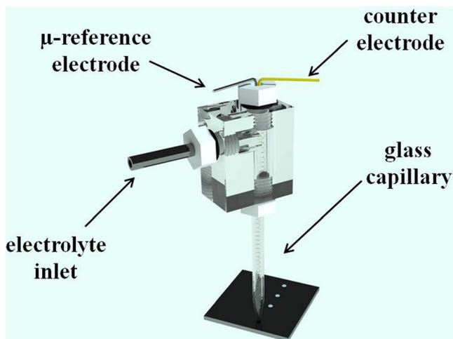
**Fig. 2** Schematic drawing of the SDCM setup used for selective dissolution of the NiAl matrix
