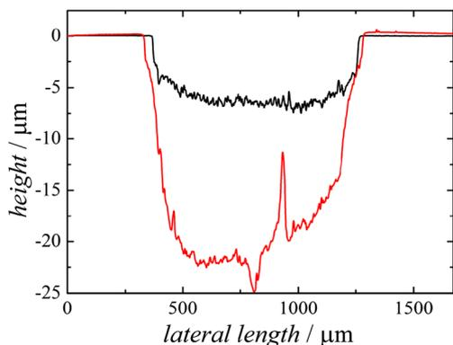
**Fig. 5** Depth profiles of two typical microvials for a dissolution time of 100 s (black line) and 300 s (red line) obtained by profilometry
