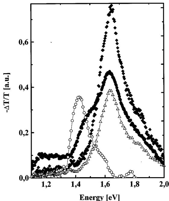
FIG. 11.  $-\Delta T/T$  for PS/MEH-PPV samples with intermediate  $C_{60}$  pumped at 488 nm [full circles (●)] and at 354 nm [full karo (◆)] at 80 K and  $10^{-5}$  Torr. For better comparison the two reference systems, PS/MEH-PPV [hollow circles (○)] and PS/ $C_{60}$  [hollow triangles (△)] are included.
