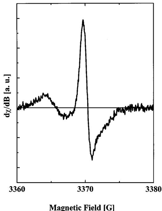
FIG. 14. LESR spectrum [full line (—)] of the concentrated PS/MEH-PPV/PC<sub>61</sub>BM compound with equal weight ratios. LESR spectrum is recorded under identical conditions as the PS/MEH-PPV/C<sub>60</sub> sample as the difference between the illuminated signal and the signal after switching off the light. Microwave power is 0.2 mW.
