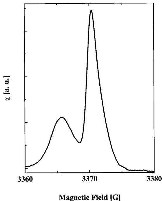
FIG. 15. Integral of LESR spectrum [full line (—)] of the concentrated PS/MEH-PPV/PC<sub>61</sub>BM compound presented in Fig. 14. Evaluation of the signal yields two peaks at identical  $g$  values as for the PS/MEH-PPV/C<sub>60</sub> sample at  $g = 2.0023$  and at  $g = 1.9997$ . Therefore peaks are interpreted as MEH-PPV<sup>+</sup> polaron and PC<sub>61</sub>BM<sup>-</sup> anion, respectively.
