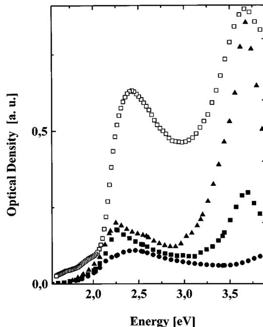
FIG. 3. Absorption data of PE/MEH-PPV/PC<sub>61</sub>BCR and PS/MEH-PPV composites with different concentrations of C<sub>60</sub> at room temperature. Spectra have been recorded from free standing films. The notation of the curves is: empty squares (□) PE/MEH-PPV/PC<sub>61</sub>BCR, full circles (●) PS/MEH-PPV, full squares (■) PS/MEH-PPV/low C<sub>60</sub> and full triangles (▲) PS/MEH-PPV/high C<sub>60</sub>.
