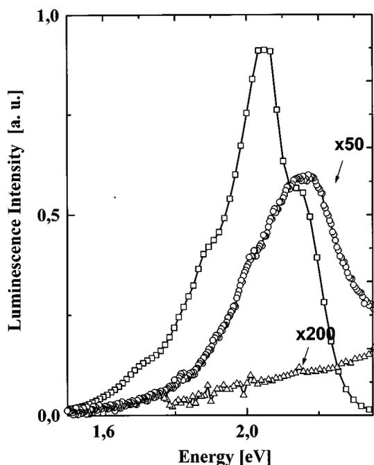
FIG. 6. Luminescence measurements of PS/MEH-PPV samples with different concentrations of  $C_{60}$  at 80 K and  $10^{-5}$  Torr. The notation of the curves is: hollow squares ( $\square$ ) PS/MEH-PPV, hollow circles ( $\circ$ ) PS/MEH-PPV/low  $C_{60}$  (scaled 50 times) and hollow triangles ( $\triangle$ ) PS/MEH-PPV/high  $C_{60}$  (scaled 200 times).
