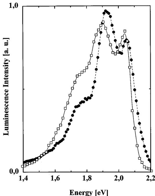
FIG. 4. Luminescence data of PE/MEH-PPV composites with [hollow squares (□)] and without [full circles (●)] PC<sub>61</sub>BCR at 80 K and 10<sup>-5</sup> Torr. The weight ratio between MEH-PPV and PC<sub>61</sub>BCR is 1:2. For the oriented sample the 488 nm pump beam is parallel to the stretch direction.
