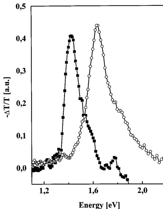
FIG. 7.  $-\Delta T/T$  for PS/MEH-PPV [full squares ( $\blacksquare$ )] and PS/ $C_{60}$  [hollow circles ( $\circ$ )] composite at 80 K and  $10^{-5}$  Torr. The energetic position of the PS/MEH-PPV peak is at 1.41 eV, the peak of the PS/ $C_{60}$  system is at 1.63 eV.
