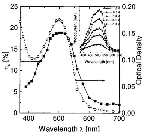
FIG. 7. Spectral resolved photon to carrier conversion efficiency  $\eta_c$  of a MDMO-PPV-PCBM (1:3) device.  $\eta_c$  was calculated according to Eq. (3). The inset shows the spectral resolved photocurrent under four different voltages (-1, -0.5, 0.5, and 1 V) and at short circuit conditions.
