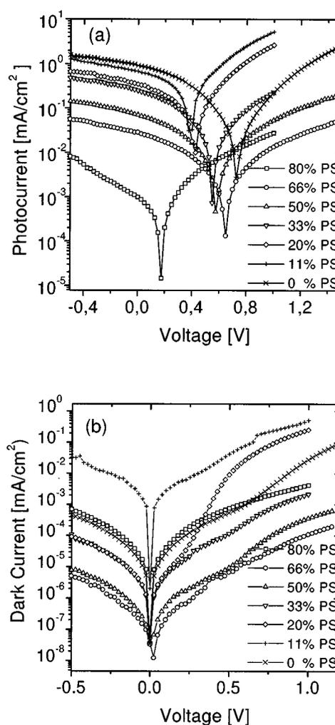
FIG. 4. (a) Short circuit current  $I_{sc}$  of various PS-MDMO-PPV-PCBM devices vs applied voltage with the concentrations denoted. Samples were measured under a vacuum better than  $10^{-5}$  mbar when illuminated by  $10 \text{ mW/cm}^2$  at 488 nm by a defocused Ar laser beam. (b) Dark current vs applied voltage for the PS-MDMO-PPV-PCBM devices with the concentrations denoted.
