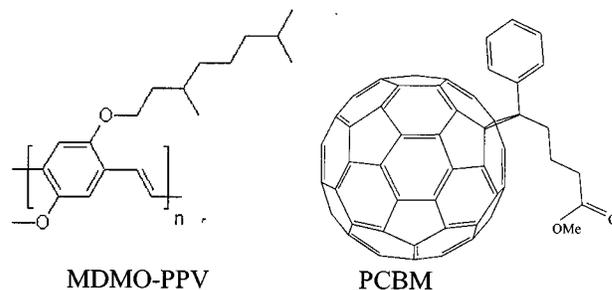
FIG. 1. Chemical structure of MDMO-PPV and PCBM.
