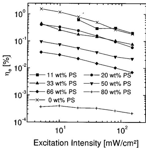
FIG. 6. Power efficiency  $\eta_e$  of various PS-MDMO-PPV-PCBM cells vs excitation intensity. Lines are drawn as a guide to the eye. Excitation is provided by Ar<sup>+</sup> laser at 488 nm.
