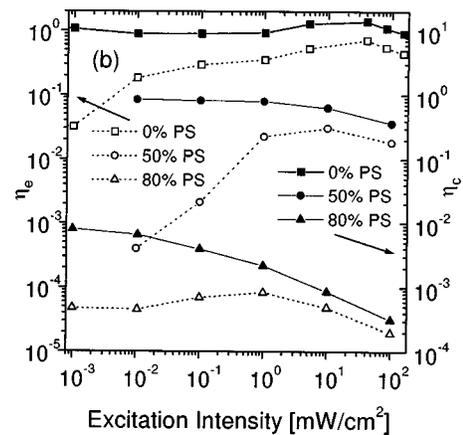
FIG. 8. (a) Carrier conversion efficiency  $\eta_c$  for three devices with 0%, 50%, and 80% PS. Data for the 50% and 80% device are multiplied by a factor 50 and 5000, respectively. (b) Excitation intensity dependence of  $\eta_e$  (left axis, open symbols) as well as  $\eta_c$  (right axis, full symbols) for devices with 0%, 50%, and 80% PS. Excitation is provided by defocused Ar<sup>+</sup> laser beam at 488 nm with neutral density filters.
