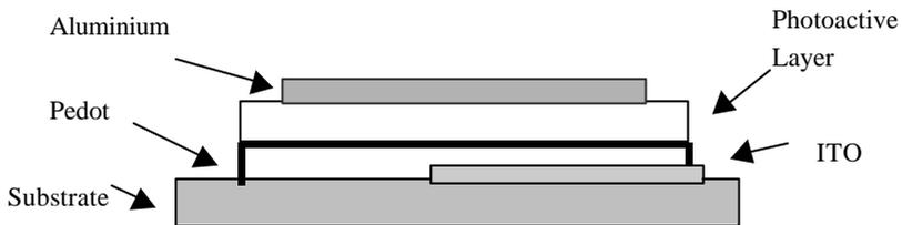
*Figure 1. Device structure*
