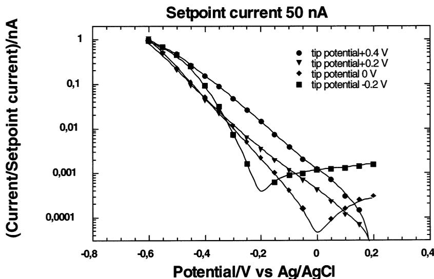
Fig. 7. Semilogarithmic plot of the normalized current through the tunneling tip measured in 0.01 M H<sub>2</sub>SO<sub>4</sub> for a setpoint current of 50 nA and different tip potentials.
