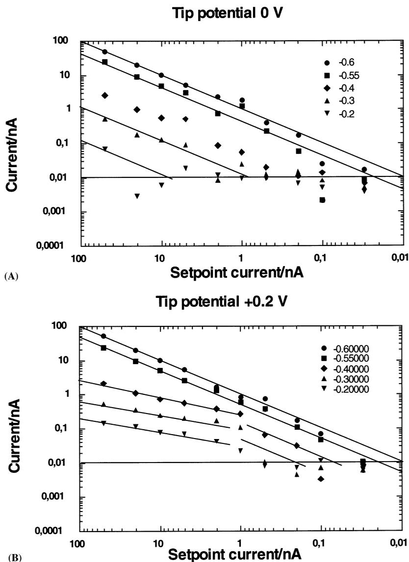
Fig. 8. Logarithmic plot of the tunneling current through the tip measured in 0.01 m  $\text{H}_2\text{SO}_4$  plotted versus the setpoint currents for different semiconductor potentials and a tip potential of (a) 0 V; (b)  $+0.2$  V; (c)  $+0.4$  V; and (d)  $-0.2$  V.
