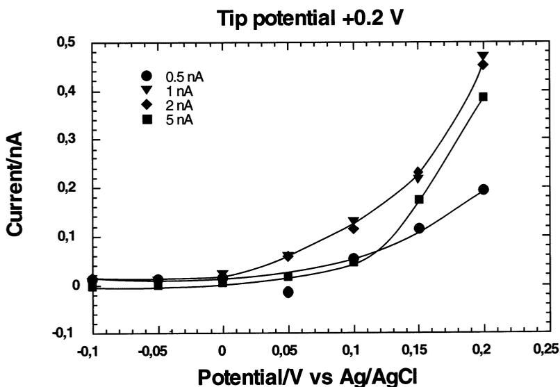
Fig. 9. Plot of the tunneling current through the tip vs. the semiconductor potential for different setpoint currents and a tip potential of +0.2 V in 0.0 1 m H<sub>2</sub>SO<sub>4</sub>.
