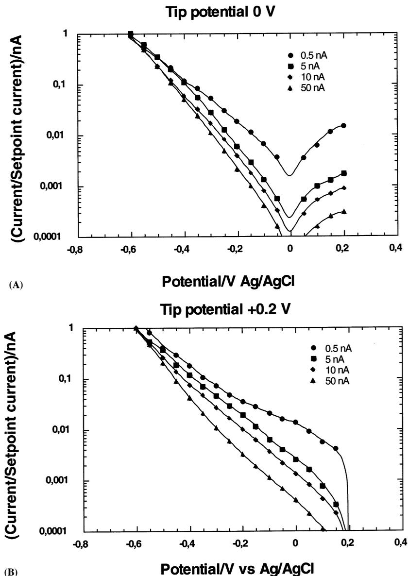
Fig. 6. Semilogarithmic plot of the normalized current through the tunneling tip versus the semiconductor potential, measured in 0.01 M H<sub>2</sub>SO<sub>4</sub> recorded for different setpoint currents with a tip potential of (a) 0 V; (b)  $+0.2$  V; (c)  $+0.4$  V; and (d)  $-0.2$  V.
