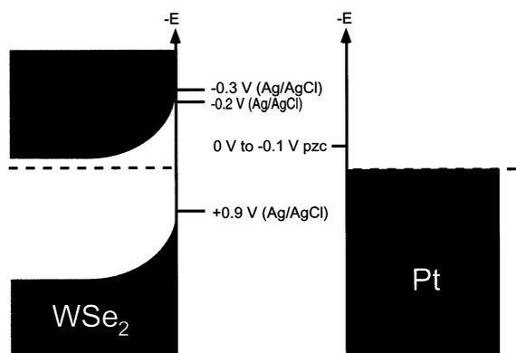
Fig. 5. Energy levels of the band edges of *n*-WSe<sub>2</sub> (left side) and the Fermi level as well as the pzc of the platinum tip (right side) in solution.
