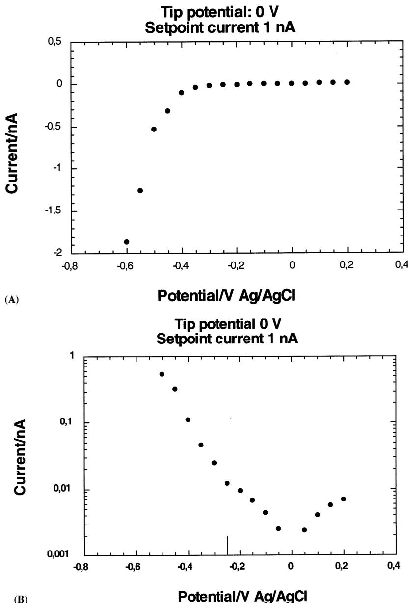
Fig. 4. Current–voltage behavior measured with a tip potential of 0 V versus Ag/AgCl and a setpoint current of 1 nA in 0.01 M  $\text{H}_2\text{SO}_4$ : (a) linear plot of the current between the tunneling tip and the sample; (b) semilogarithmic plot of the current through the tunneling tip.
