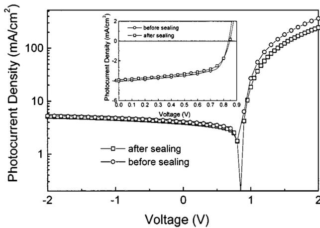
FIG. 3. Typical  $I$ - $V$  curves for an "as-produced" polymer-fullerene solar cell before and after sealing. Measurements were performed with a solar simulator (Steuernagel solar constant 575) at an irradiance level of  $800 \text{ W/m}^2$  and a cell temperature of  $55^\circ\text{C}$ . Measured data were corrected to the plotted AM1.5 values using a calculated (Ref. 17) mismatch factor of 0.76.
