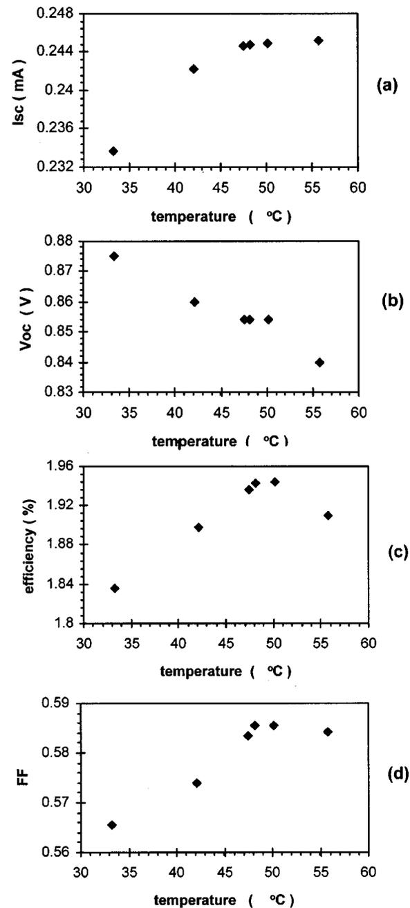
FIG. 4. Temperature dependencies of the principal photovoltaic parameters for a typical polymer-fullerene solar cell derived from outdoor measurements of its  $I$ - $V$  curves. Plotted values of efficiency and  $I_{sc}$  have been adjusted to the STC irradiance level of  $1000 \text{ W/m}^2$ .
