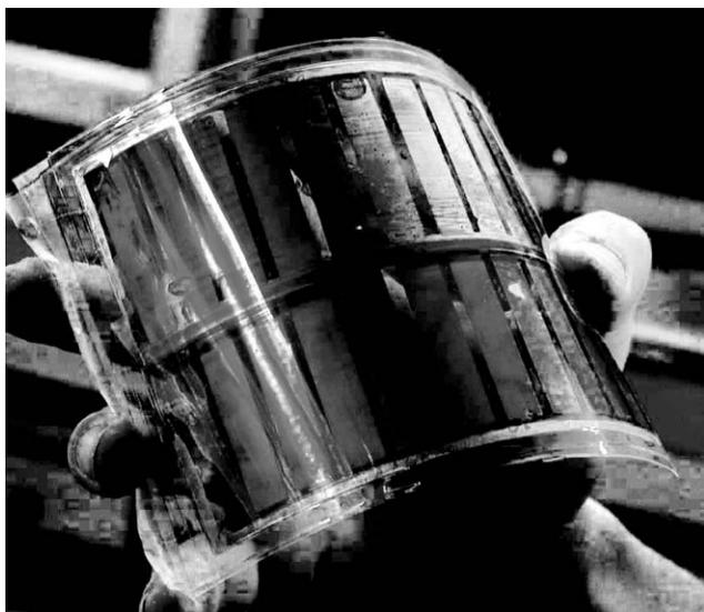
Fig. 3 Picture of a large area flexible plastic solar cell. (Reproduced with permission of WILEY-VCH.)
