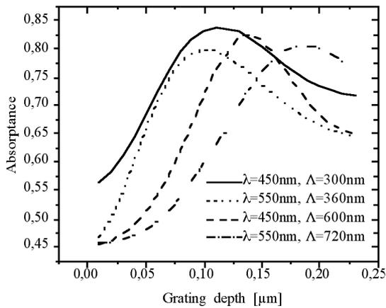
**Figure 7:** Absorbance versus the grating depth for the 1<sup>st</sup> and 2<sup>nd</sup> order coupling at the wavelengths 450nm and 550nm.
