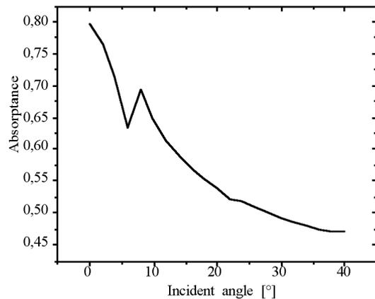
**Figure 9:** Absorbance versus the incident angle ( $\lambda=550\text{nm}, \Lambda=360\text{nm}, \text{Grating depth} = 110\text{nm}$ )
