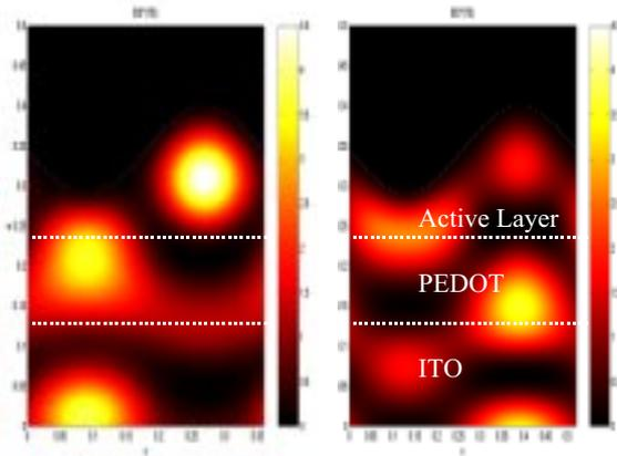
**Figure 5:** Near-field intensity  $EE^*$  in the cross section for the cell with  $\Lambda=360\text{nm}$  (Situation A of Figure 4)
