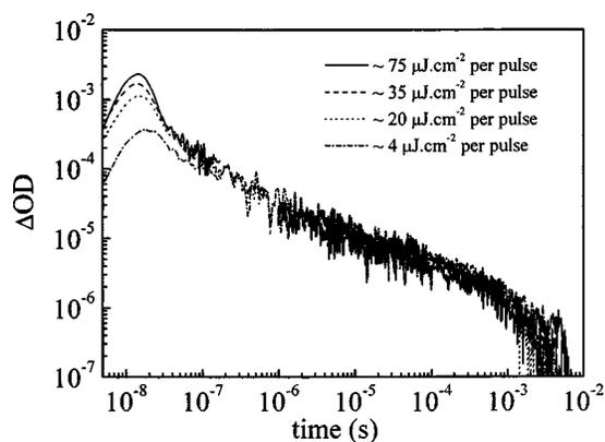
FIG. 4. Transient absorption decay kinetics observed for the MDMO-PPV/PCBM blend on the nanosecond to millisecond time scales. Transient absorption data for time delays  $>300$  ns collected at 940 nm. Other experimental conditions as for Fig. 2.
