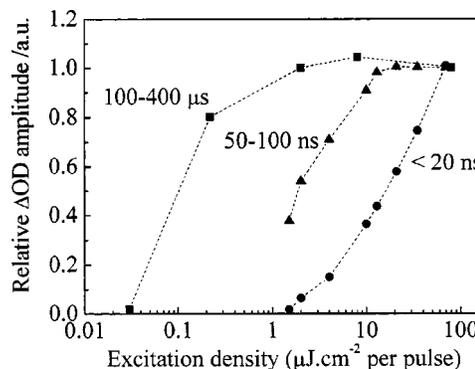
FIG. 3. Relative amplitude of the transient absorption signal for the MDMO-PPV/PCBM blend as a function of laser excitation power: (—●—) amplitude of instrument response ( $\sim 20 \text{ ns}$ ) limited decay; (---▲---) transient signal at 50–100 ns; (---■---) transient signal at 100–400  $\mu\text{s}$ . Other experimental conditions as for Fig. 2.
