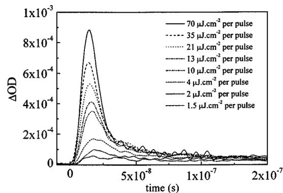
FIG. 2. Transient absorption kinetics observed for the MDMO-PPV/PCBM blend on the nanosecond time scale using different excitation densities. The excitation densities ranged between 1.5 and  $70 \mu\text{J cm}^{-2}$  per pulse. The decay is assigned to charge recombination between electrons in the fullerene and the positive polarons in the conjugated polymer. The sample was excited at 500 nm at a repetition rate of 4 Hz and probed using a laser diode at 830 nm,  $T = 296 \text{ K}$ .
