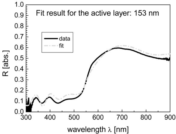
**FIGURE 5** Measured (full line) and fitted (dash-dots) reflection spectra of a complete solar cell structure illuminated from the glass side. The only fit parameters were the layer thicknesses of ITO, PEDOT:PSS and of the MDMO-PPV:PCBM layer.
