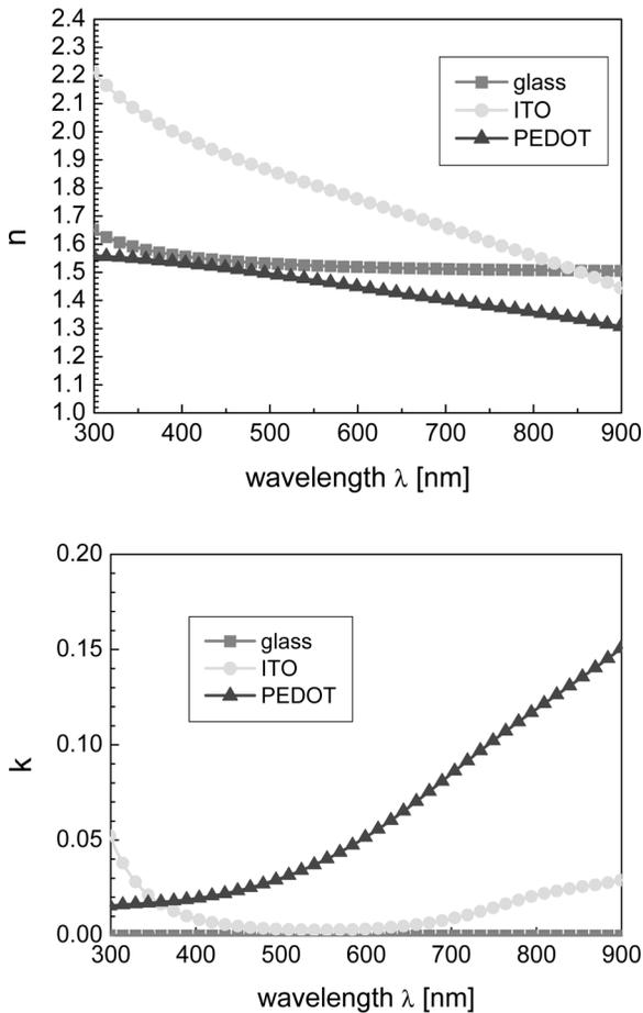
**FIGURE 3** Optical constants of the ITO-substrate glass (triangles), the ITO (circles) and the PEDOT:PSS (squares) layer, determined by fitting model dielectric functions to the respective transmission and reflection data.
