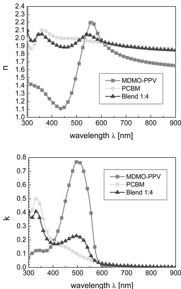
**FIGURE 4** Optical constants of pristine MDMO-PPV (squares), PCBM (circles) and the MDMO-PPV:PCBM 1:4 blend, determined by fitting model dielectric functions to the respective transmission and reflection data of single layer films on fused silica.
