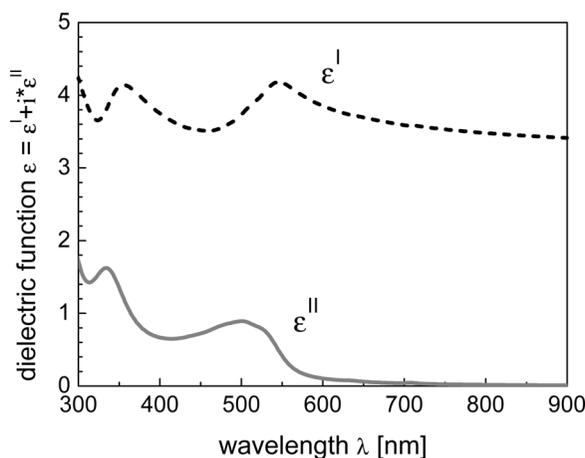
**FIGURE 2** Real ( $\epsilon'$ ) and the imaginary part ( $\epsilon''$ ) of the model dielectric function of the MDMO-PPV:PCBM 1:4 blend in a 110 nm thick film spin cast from a chloro-benzene solution 1,4% by weight.
