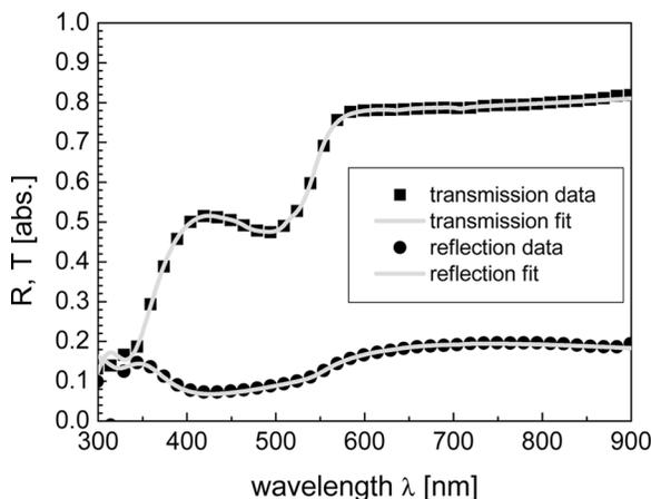
**FIGURE 1** Measured and fitted transmission and reflection spectra of a thin film of the MDMO-PPV:PCBM mixture (1:4 weight ratio), spin coated from chloro-benzene solution onto fused silica substrates.
