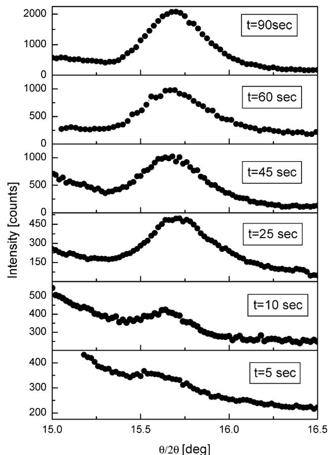
Fig. 3.  $\theta/2\theta$ -scans of the (1 1  $\bar{1}$ ) reflection of PSP for different growth times. The growth temperature was  $150^\circ\text{C}$ .
