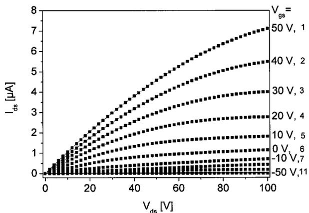
FIG. 2. Transistor characteristics of an OFET with channel length  $L=65 \mu\text{m}$ , channel width  $W=1.4 \text{ mm}$  for different  $V_g$ . All measurements were carried out at room temperature. The data shown here are taken in descending  $V_g$  mode from 50 to  $-50 \text{ V}$  in steps of  $10 \text{ V}$  as labeled from 1 to 11. The integration time is 1 s.
