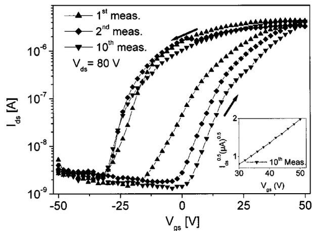
FIG. 3. Transfer characteristics of the OFET with  $V_{\text{ds}}=80 \text{ V}$  demonstrating the nonvolatile organic memory device. Each measurement was carried out with an integration time of 1 s. Inset:  $I_{\text{ds}}^{0.5}$  vs  $V_{\text{gs}}$  plot for the tenth measurement.
