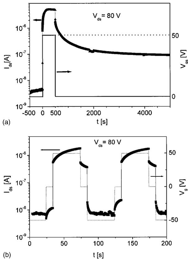
FIG. 4. (a) Logarithmic  $I_{ds}$  vs time ( $t$ ) plot at  $V_{ds}=80$  V for floating gate (denoted by  $V_g=0$  V), during  $V_g=50$  V and floating gate sequentially showing long retention time. The data were taken each 250 ms and every second data point is plotted. (b) Switching response of the drain current, upon application of gate voltage pulses with a pulse height of  $\pm 50$  V and a pulse duration of 40 s.
