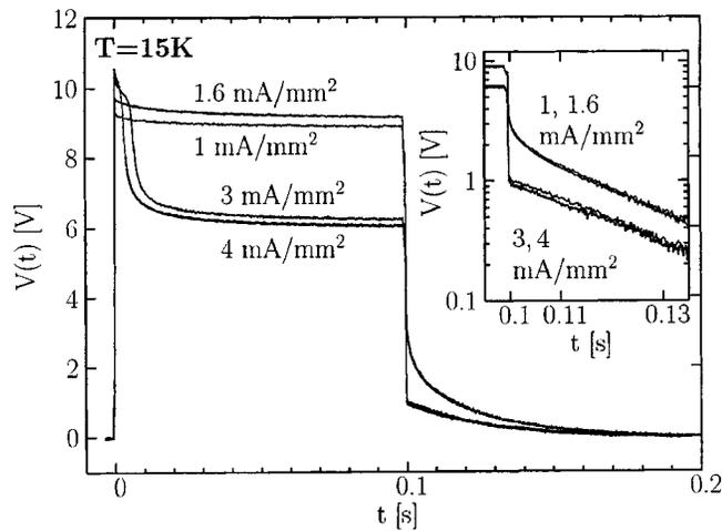
FIG. 4. Low temperature ( $T=15$  K), time-resolved voltage response  $V(t)$  for a 100 ms current pulse with various injected current densities. At  $t=0$ , the current density is set to 1, 1.6, 3, and 4  $\text{mA}/\text{mm}^2$ , respectively, and at  $t=0.1$  s it is set back to zero. The inset displays a magnified part of the voltage response on a logarithmic voltage scale around the end of the current pulse at  $t=0.1$  s.
