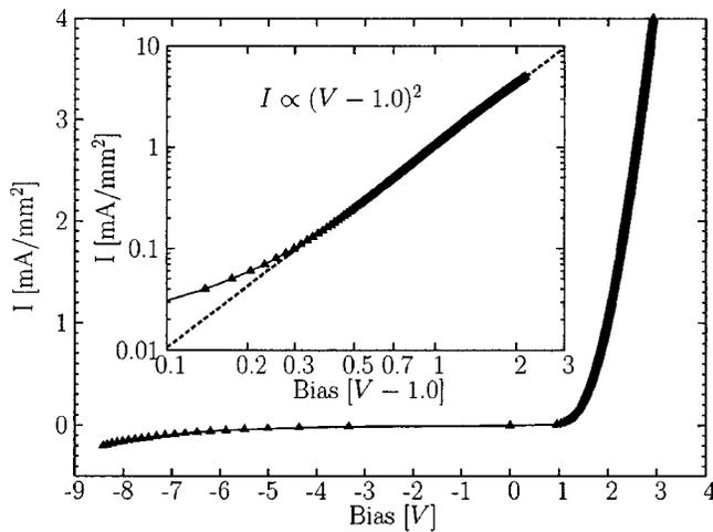
FIG. 2. Room temperature  $V$ - $I$  characteristic of ITO/PEDOT:PSS/PCBM device with LiF/Al/Au (0.7/70/100 nm) top contact. Above 1 V, effective charge injection takes place. The injected electron current is SCLC as evidenced by the quadratic dependency vs the effective measured bias  $V - V_{bi}$  shown in the inset.
