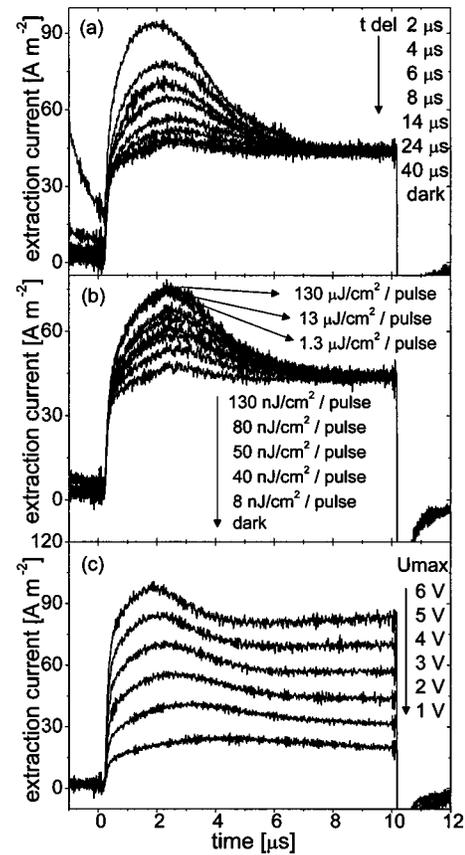
FIG. 2. Measured Photo-CELIV curves at (a) various delay times ( $t_{\text{del}}$ ) between the light pulse and the voltage pulse; (b) various incoming light intensity at fixed  $t_{\text{del}} = 5 \mu\text{s}$ ; and (c) various  $U_{\max}$ .
