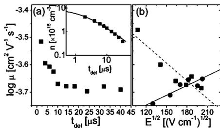
FIG. 3. Photo-CELIV mobility as a function of delay time (a) and the electric field (b) at (■) 5  $\mu\text{s}$  or (●) 15  $\mu\text{s}$  after the light pulse. Inset: Concentration of extracted charge carriers as function of delay time and the fit.
