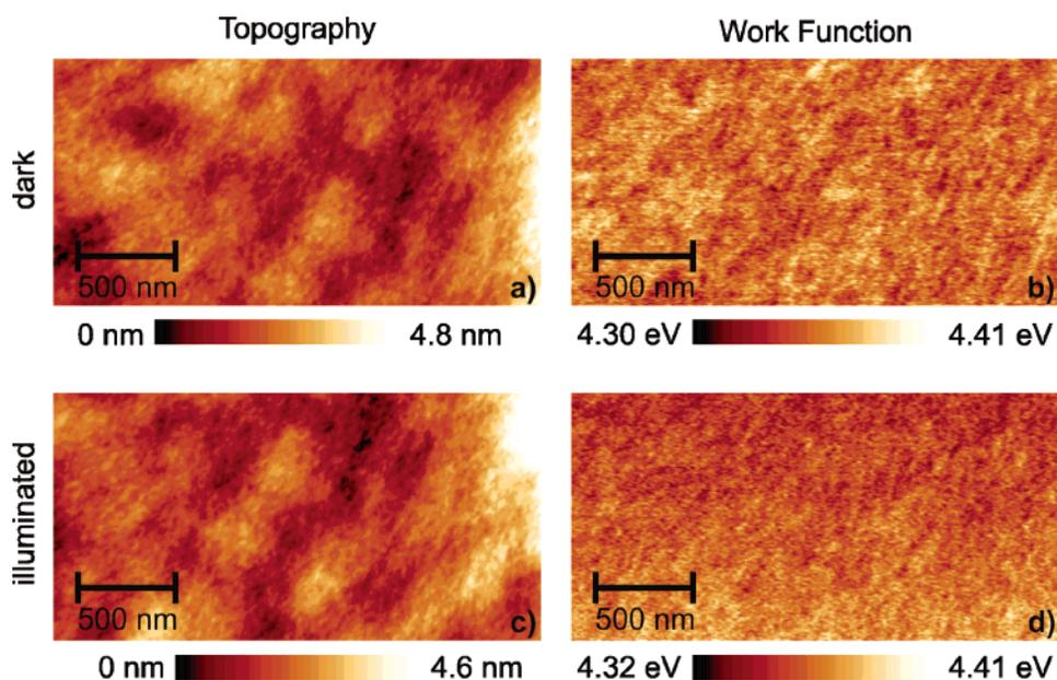
**Figure 2.** Topography (a, c) and work function (b, d) of a pristine PCBM film in the dark (a, b) and under 442 nm HeCd laser illumination (c, d).
