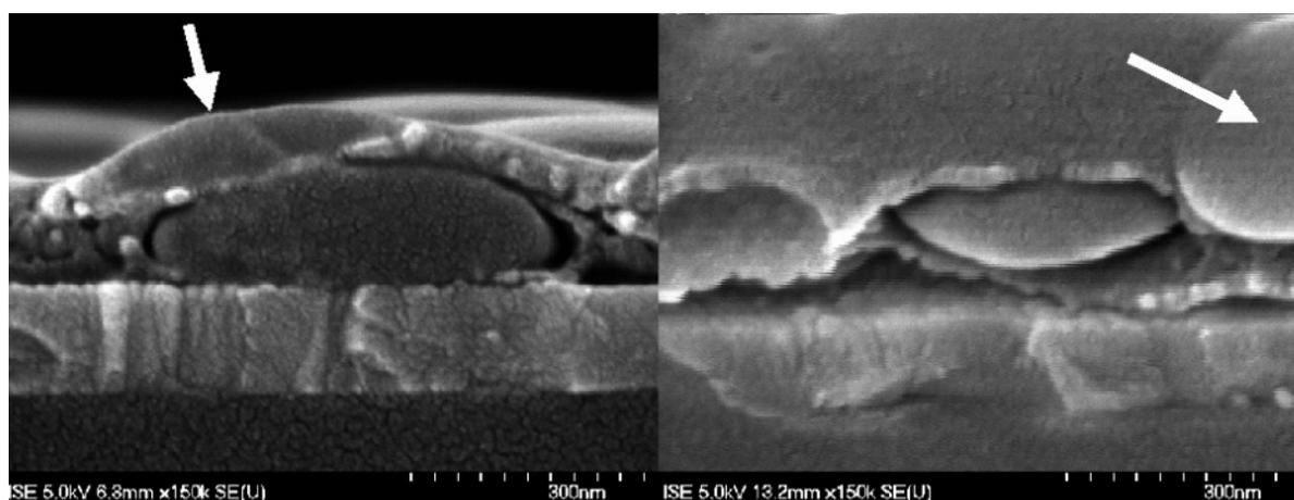
**Figure 6.** Cross-sectional SEM images of toluene-cast MDMO-PPV/PCBM blend films. The white arrows point to regions where PCBM clusters are exposed freely to the surface of the film.
