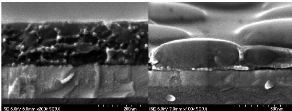
**Figure 5.** SEM measurements on cross sections of MDMO-PPV/PCBM 1:4 blends. On the left a chlorobenzene- and on the right a toluene-cast film are shown for comparison. Polymer nanospheres (brighter) are rather evenly distributed in the film on the left, while they surround the large PCBM clusters as a “skin-layer” in the right.<sup>23</sup>
