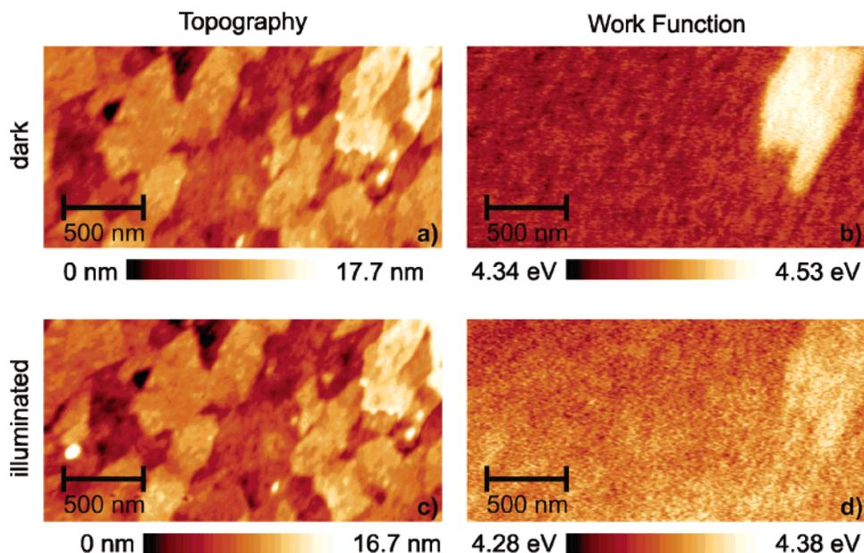
**Figure 1.** Topography (a, c) and work function (b, d) of a pristine MDMO-PPV film in the dark (a, b) and under 442 nm HeCd laser illumination (c, d).
