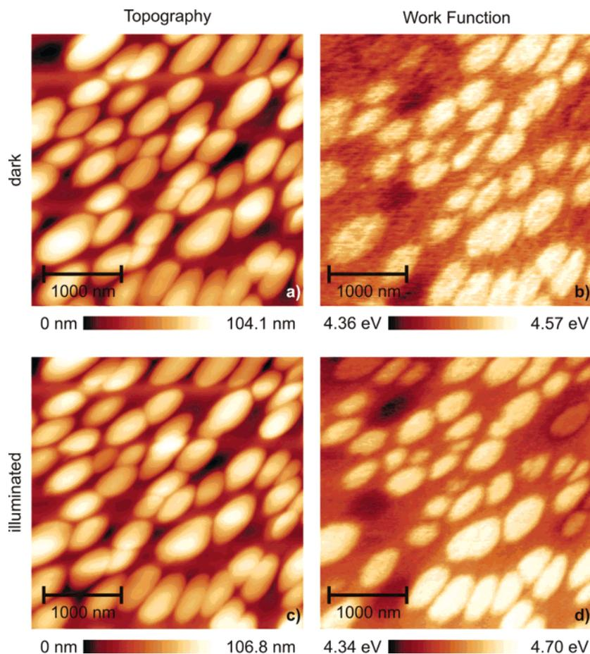
**Figure 4.** Topography and work function of a toluene-cast blend film of MDMO-PPV/PCBM with a mass ratio of 1:4, measured in the dark and under 442 nm cw laser illumination. Note that some of the topographical hills lead to dark areas and thus low work functions, whereas the majority of the hills result in bright areas with high work functions.
