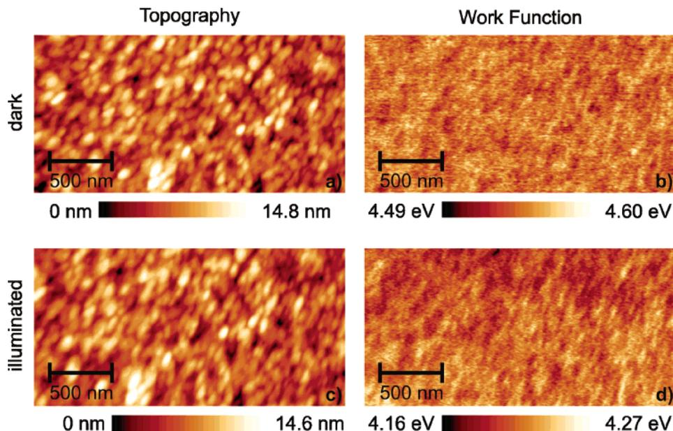
**Figure 3.** Topography (a, c) and work function (b, d) of a chlorobenzene-cast blend film of MDMO-PPV/PCBM with a mass ratio of 1:4, measured in the dark (a, b) and under 442 nm cw laser illumination (c, d).
