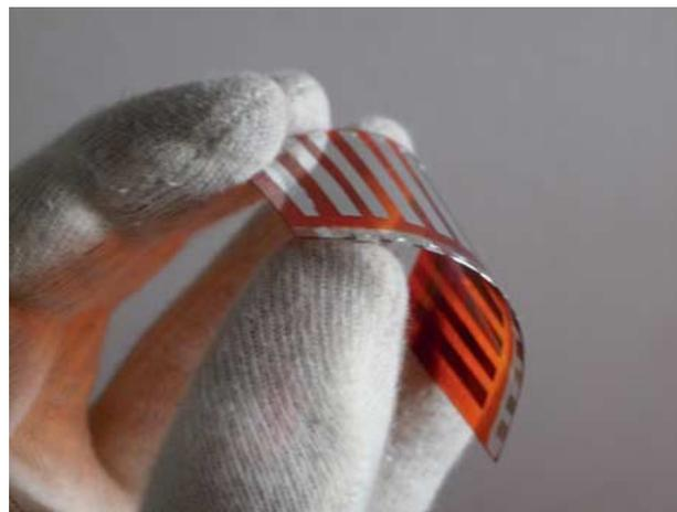
**Fig. 8.** Picture of a flexible  $6.5 \times 4.1 \text{ cm}^2$  MDMO-PPV:PCBM solar cell realized on a PET substrate.
