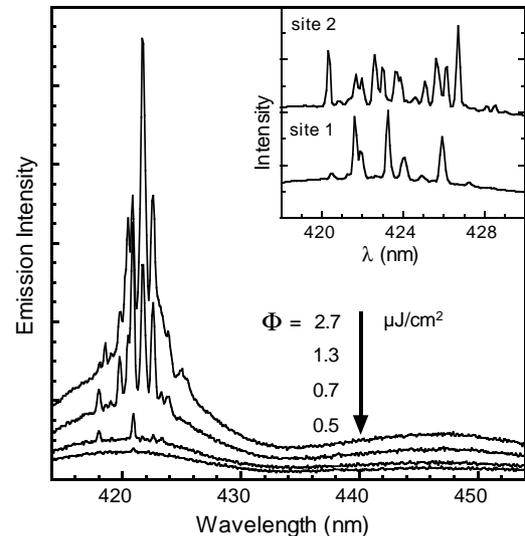
Fig. 2. Emission spectra taken at different values of the pump fluence  $\Phi$  ( $\mu\text{J}/\text{cm}^2$  per pulse). Inset: Emission spectra measured in two different positions across the sample surface at the same excitation level above threshold.
