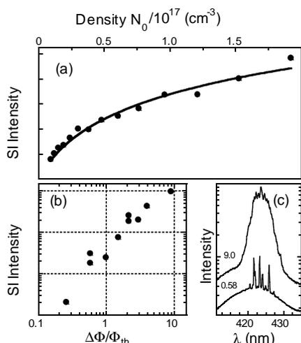
Fig. 3. (a) Spectrally integrated (SI) emission intensity vs photoexcited density  $N_0$ , for pump intensities below threshold. (b) Spectrally integrated pump excess fluence  $\Delta\Phi/\Phi_{th}$ . (c) Emission spectra recorded at  $\Delta\Phi/\Phi_{th} = 0.58$  and 9.0.
