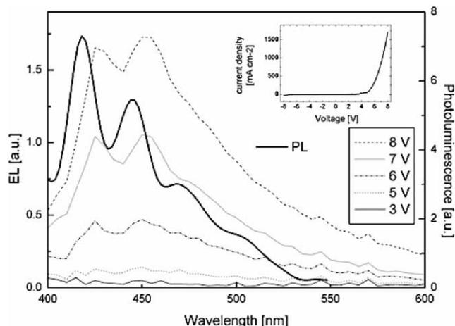
Fig. 4. Electroluminescence of a PSP ( $d = 100$  nm) single device at different voltage. Inset shows the corresponding current–voltage curve. Full line shows the photoluminescence of a PSP film on mica.
