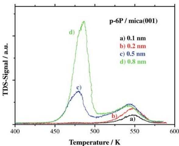
**FIGURE 6** Thermal desorption spectra for p-6P on mica(001). Adsorption temperature 360 K, heating rate 1 K/s. The mean thickness of the individual films as measured with the quartz microbalance is indicated
