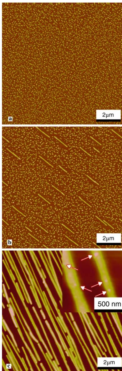
**FIGURE 1** Different growth stages of p-6P films on mica. Pure island growth after 30 sec (a); islands (crystallites) and chains after 45 sec (b); long term growth morphology after 9 min, consisting only of chains (c). The inset in (c) shows a higher resolution scan, revealing that in this stage small crystallites are formed on top of the chains. z-scale for all pictures is 50 nm
