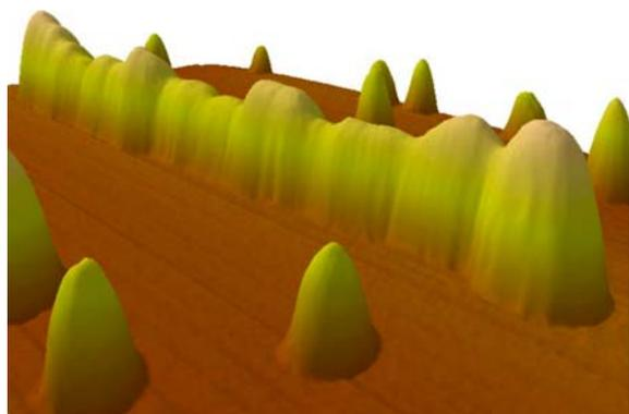
**FIGURE 2** Detailed 3D-image of a single 850 nm long chain after 35 seconds of p-6P deposition (intermediate stage) revealing the interior structure of the chain.  $1 \times 1 \mu\text{m}$  scan,  $z$ -scale is 30 nm
