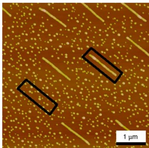
**FIGURE 5** AFM image revealing denuded zones around chains. The amount of material in the lower rectangle is approximately equal to the amount of material needed to build the chain in the upper rectangle. z-scale is 50 nm
