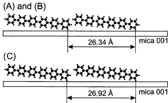
FIG. 3. Side view of *p*-6P molecules relative to the mica (001) substrate as they are oriented within their epitaxial orientations. Top part: Orientations (A) and (B) with the same intermolecular distance of  $a=26.34$  Å. Bottom part: Orientation (C) with another distance of  $a=26.92$  Å.
