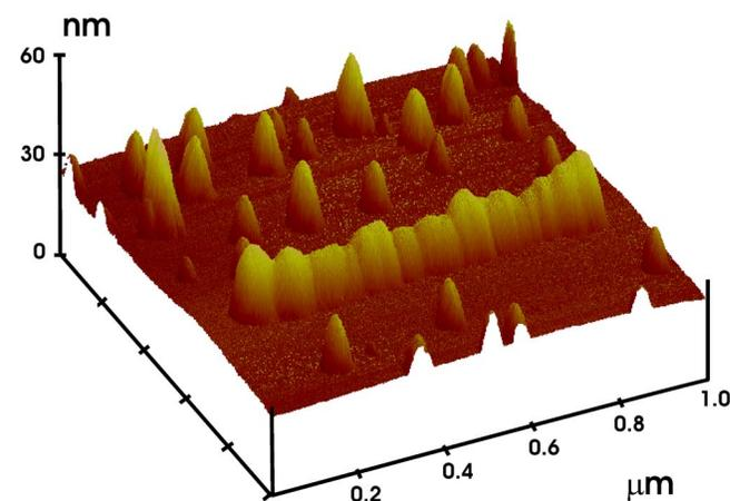
FIG. 2. (Color online) High-resolution three-dimensional AFM image showing individual *p*-6P islands as well as a single nanofiber.
