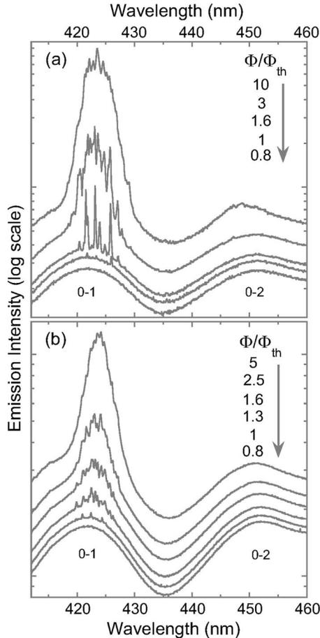
FIG. 5. (a) Room-temperature emission spectra of the *p*-6P nanofibers with  $\langle h \rangle \approx 110$  nm (sample *E*) for different values of the pump fluence  $\Phi/\Phi_{th}$  ( $\Phi_{th} \approx 1 \mu\text{J}/\text{cm}^2$  per pulse). (b) Same as in panel (a) but measured in the sample with  $\langle h \rangle \approx 290$  nm (sample *F*,  $\Phi_{th} \approx 6 \mu\text{J}/\text{cm}^2$ ).
