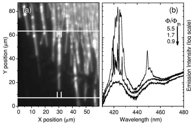
FIG. 6. (a) Gray-scale micrograph of random lasing nanofibers (sample *E*). The excitation fluence is  $\approx 60 \mu\text{J}/\text{cm}^2$  per pulse. The white markers are delimiters for the area over which the spectra shown in (b) are spatially integrated. (b) Emission spectra measured for different values of the pump fluence  $\Phi/\Phi_{\text{th}}$  ( $\Phi_{\text{th}} \approx 35 \mu\text{J}/\text{cm}^2$ ).
