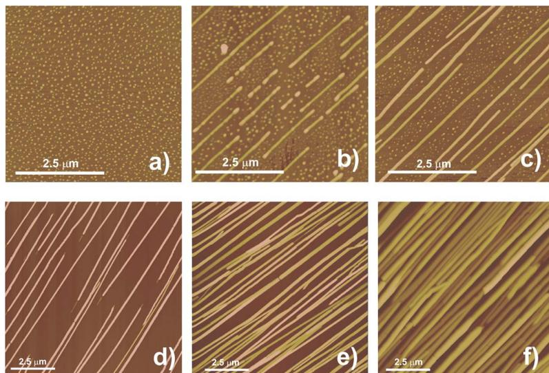
FIG. 1. (Color online) AFM topography images of the *p*-6P films grown within (a) 10 s, (b) 25 s, (c) 90 s, (d) 5 min, (e) 40 min, and (f) 120 min. The growth temperature was 130 °C. The Z scale is 0–50 nm in (a)–(c), 0–100 nm in (d), 0–220 nm in (e), and 0–700 nm in (f).
