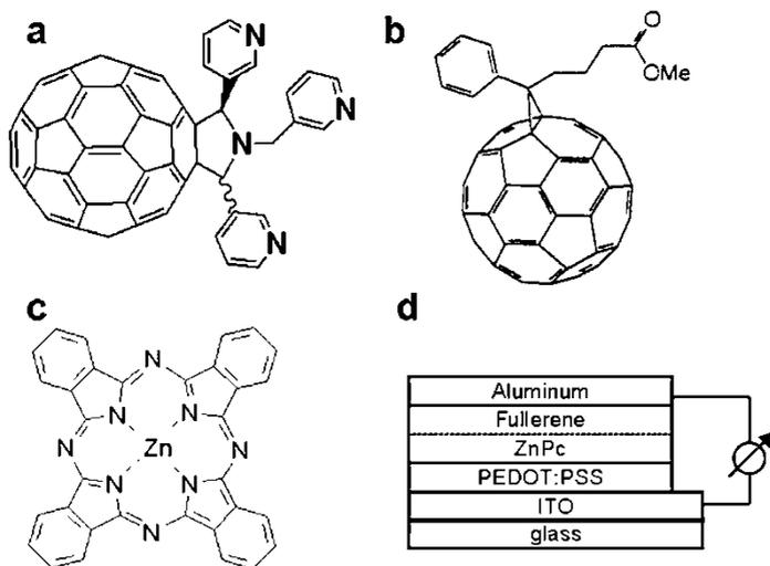
**Figure 1.** Structure formulae of the materials used in this study: (a) pyrrolidinofullerene bearing three chelating pyridyl groups (PyF); (b) 1-(3-methoxycarbonyl) propyl-1-phenyl [6,6] C<sub>61</sub> (PCBM); (c) zinc-phthalocyanine (ZnPc); (d) schematic layout of the solar cells.
