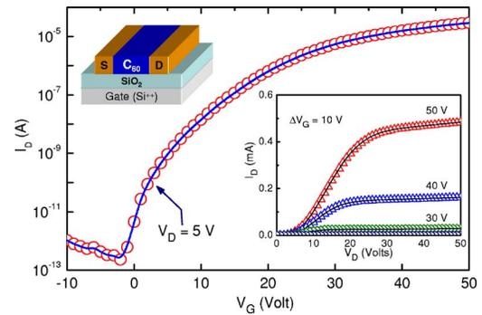
FIG. 2. (Color online) Room temperature transfer characteristic obtained from a bottom-contact C<sub>60</sub> transistor (T<sub>S</sub>=120 °C) employing SiO<sub>2</sub> as the gate dielectric. Inset diagram shows the device architecture employed. The inset figure displays the room temperature output characteristics of the transistor at different V<sub>G</sub>.
