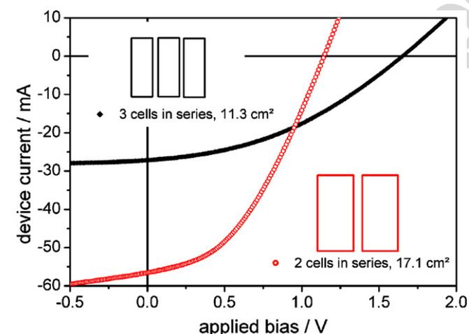
Fig. 4.  $I$ - $V$  characteristics under simulated solar irradiation of an organic, P3HT:PCBM-based solar cell module on ITO/glass substrates consisting of two (circles) or three (diamonds) cell connected in series.
