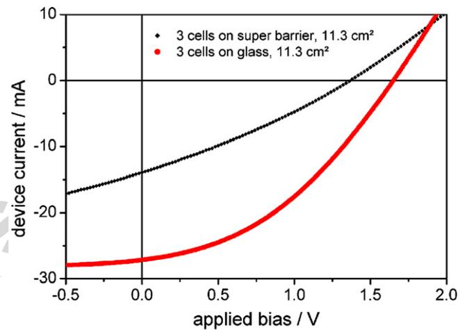
Fig. 6.  $I$ - $V$  characteristics under simulated solar irradiation of an organic, P3HT:PCBM-based solar cell module ( $11.3\text{ cm}^2$  active area) consisting of three cells connected in series on ITO/glass (circles) and ITO/ultra-high barrier substrate (diamonds).
