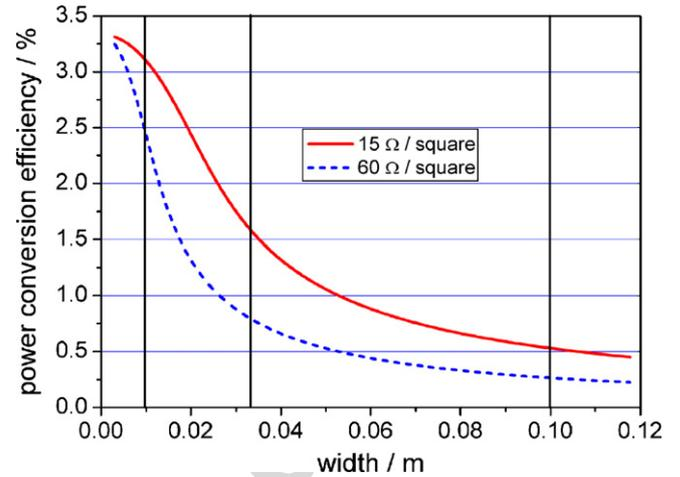
Fig. 3. Calculated theoretical power conversion efficiency of a P3HT:PCBM-based single rectangular organic solar cell as a function of the width of the electrode. Two cases are shown, an ITO sheet resistance of 15  $\Omega$ /square (solid line) and 60  $\Omega$ /square (dashed line). The vertical lines indicate the widths of the electrodes compared in Table 1.
