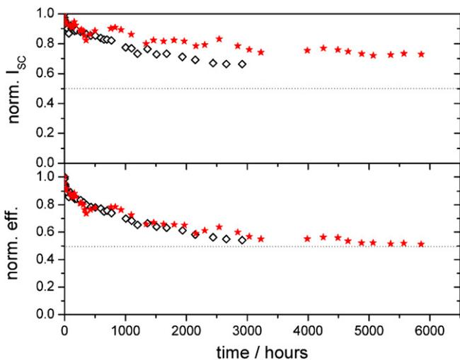
Fig. 8. Normalized  $I_{SC}$  and efficiency of solar cells based on MDMO-PPV:PCBM blends (open diamonds) and P3HT:PCBM blends (stars) encapsulated with flexible gas barrier material versus storage time in the dark under ambient air.
