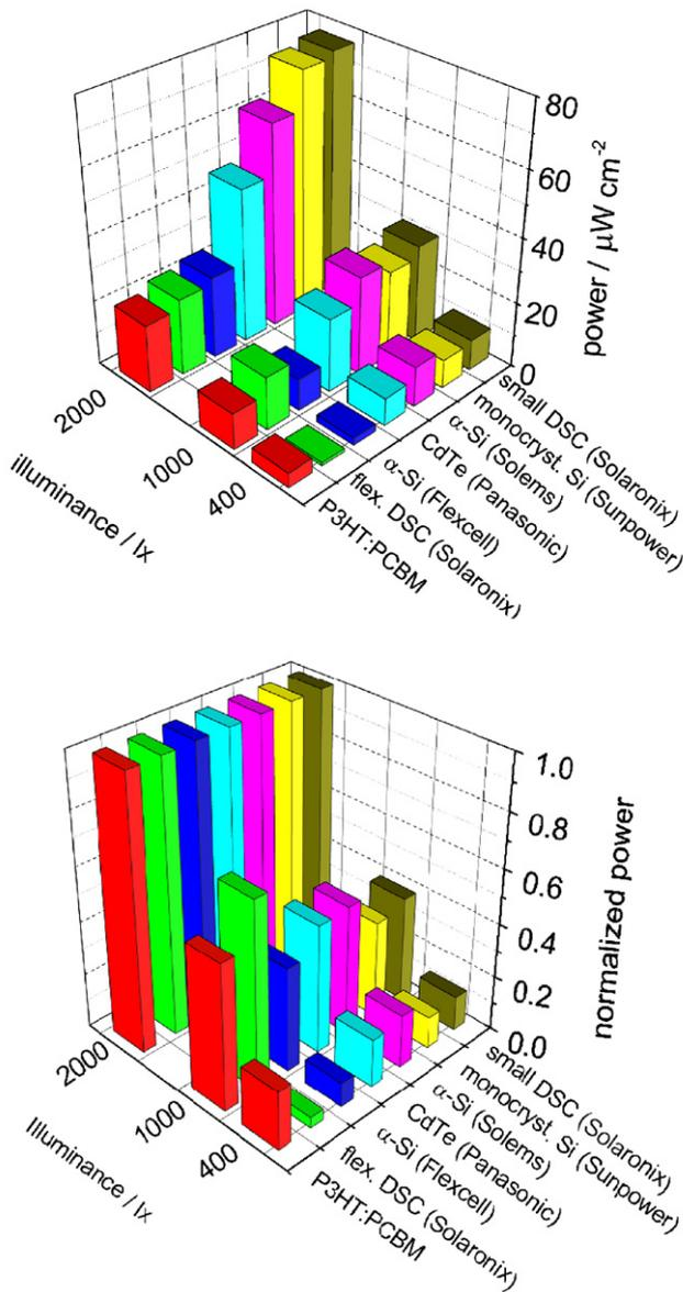
Fig. 5. Absolute (upper graph) and normalized (lower graph) power output per surface area of diverse solar cell technologies under illumination with fluorescent tubes yielding various illuminance levels.
