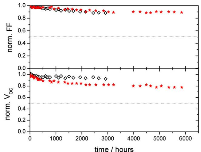
Fig. 7. Normalized  $V_{OC}$  and  $FF$  of solar cells based on MDMO-PPV:PCBM blends (open diamonds) and P3HT:PCBM blends (stars) encapsulated with flexible gas barrier material versus storage time in the dark under ambient air.
