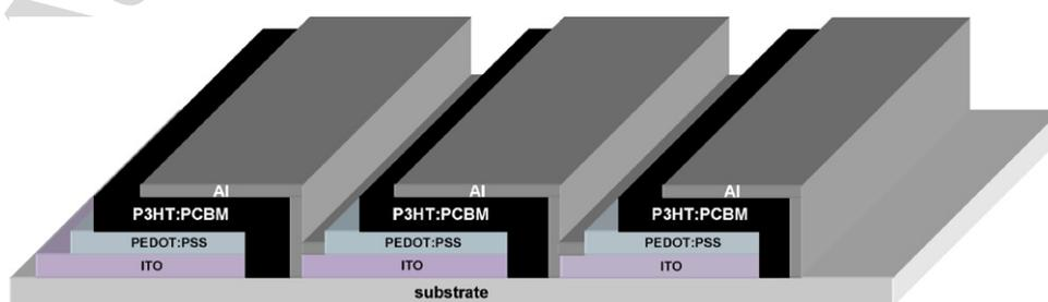
Fig. 1. Serial connection of organic solar cells.
