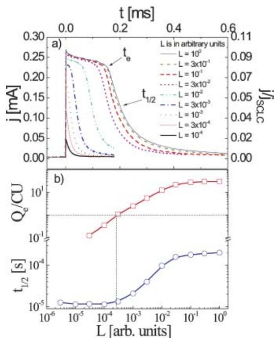
Figure 4. RRP3HT/PCBM bulk-heterojunction solar cells: experimentally measured by integral ToF transients as a function of laser light intensity in (a) and extracted charge with extraction half-time as a function of light intensity in (b). (Reprinted figure with permission from A. Pivrikas, G. Juška, A. J. Mozer, M. Scharber, K. Arlauskas, N. S. Sariciftci, H. Stubb, and R. Österbacka, *Physical Review Letters* 2005; **94**: 176806. Copyright (2005) by the American Physical Society)
