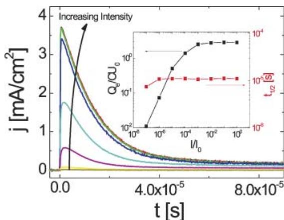
Figure 3. MDMO-PPV/PCBM bulk-heterojunction solar cells: high Intensity ToF transients, where inset shows the extracted charge and extraction half-time as a function of light intensity
