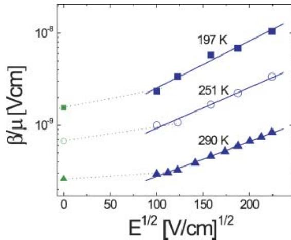
Figure 14. RRP3HT/PCBM bulk-heterojunction solar cells: ratio of the bimolecular recombination coefficient  $\beta$  with charge carrier mobility  $\mu$  as a function of electric field
