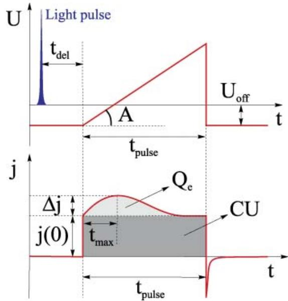
Figure 7. Applied triangle voltage pulse (top figure) and current transient response (bottom figure) in the CELIV technique.  $j(0)$  represents the displacement current, whereas  $\Delta j$  represents the current due to transported equilibrium or photogenerated charge carriers. The extracted charge  $Q_c = S \int_0^{t_{\text{pulse}}} \Delta j dt$  and  $CU = S \int_0^{t_{\text{pulse}}} j(0) dt$ , where  $S$  is the electrode area
