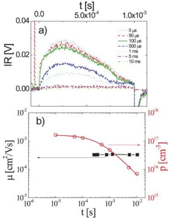
Figure 8. RRP3HT/PCBM bulk-heterojunction solar cells: current transients as a function of delay time  $t_{del}$  measured using the CELIV technique in (a) and charge carrier mobility as a function of  $t_{del} + t_{\max}$  (closed squares) plotted together with carrier concentration as a function of  $t_{del}$  in (b)
