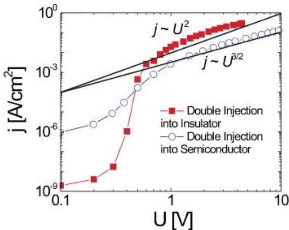
Figure 12. RRP3HT/PCBM bulk-heterojunction solar cells:  $I-V$  dependence in high and low conductivity films
