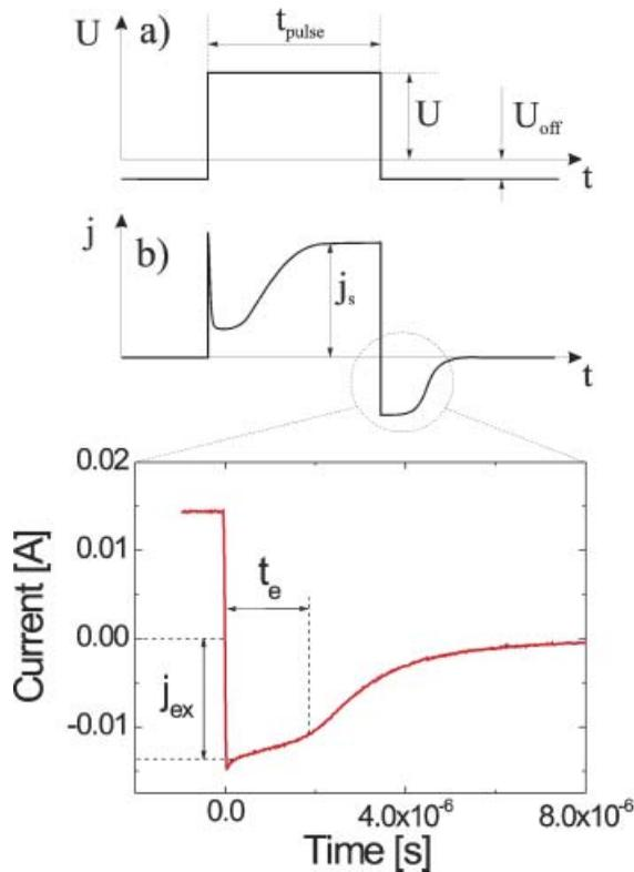
Figure 16. Plasma extraction technique: applied voltage pulse (a) and current transient response recorded in the oscilloscope (b). An experimental current transient with characteristic reservoir extraction  $t_e$  is shown in the magnified picture
