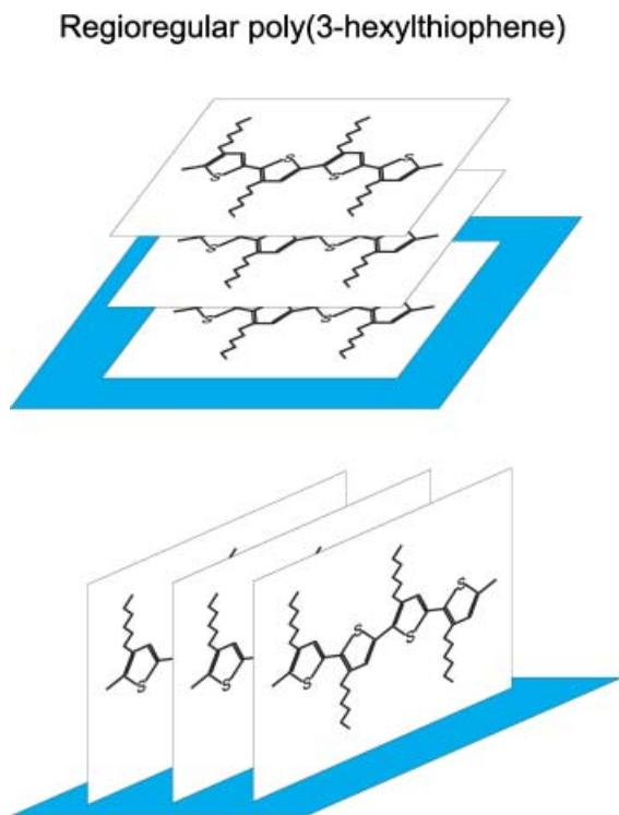
Figure 5. Two different orientations of ordered RRP3HT domains with respect to the substrate. Left picture shows horizontal stacking of RRP3HT domains, whereas right picture denotes vertical lamella stacking
