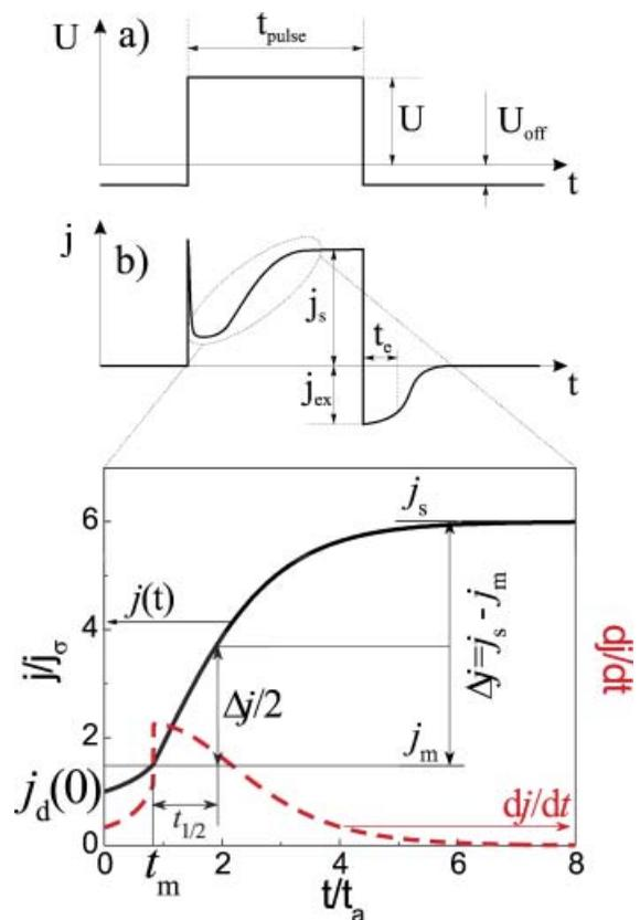
Figure 11. DI transient technique: applied voltage pulse (a) and current transient response recorded in the oscilloscope (b). An ideal DI current transient with characteristic current increase after  $RC$  spike is shown. At the end of applied voltage pulse plasma extraction time  $t_e$  is also seen in the current transient. In the magnified picture: the solid line shows the ideal DI current transient, whereas the dashed line shows the time-derivative of the DI transient
