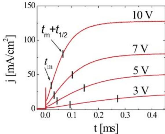
Figure 13. RRP3HT/PCBM bulk-heterojunction solar cells: DI current transients for different applied voltages. The dashes show maximum points  $t_m$  of the current derivative and  $t_m + t_{1/2}$  time used to directly calculate carrier mobility and bimolecular recombination coefficient  $\beta$  for different applied voltages
