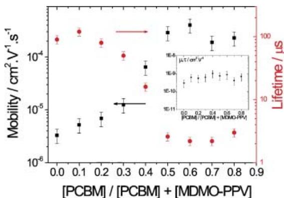
Figure 10. MDMO-PPV/PCBM bulk-heterojunction solar cells: carrier mobility  $\mu$ , lifetime  $\tau$  and  $\mu\tau$  product versus concentration ratio of the blend. (Laser intensity used in the experiment was 0.5 mJ/pulse.) (This article was published by G. Dennler, A. J. Mozer, G. Juška, A. Pivrikas, R. Österbacka, D. A. Fuchsbaauer, and N. S. Sariciftci in *Organic Electronics* 2006; 7: 229. Copyright Elsevier (2006))
