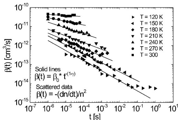
Figure 9. MDMO-PPV/PCBM bulk-heterojunction solar cells: bimolecular recombination coefficient  $\beta$  plotted as a function of time and fitted using time-dependent charge carrier mobility  $\mu$ . (Reprinted figure with permission from A. J. Mozer, G. Dennler, N. S. Sariciftci, M. Westerling, A. Pivrikas, R. Österbacka, and G. Juška, *Physical Review B* 2005; 72: 035217. Copyright (2005) by the American Physical Society)
