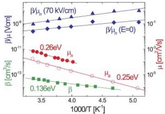
Figure 15. RRP3HT/PCBM bulk-heterojunction solar cells: electron mobility  $\mu_n$ , ambipolar carrier mobility  $\mu_a$ , bimolecular recombination coefficient  $\beta$ , and the ratio of both as a function of temperature
