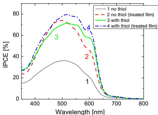
**Fig. 3.** Incident photon to current efficiency of 4 different RR-P3HT/PCBM bulk-heterojunction solar cells: as produced (thin line), annealed (thick dashed line), thiol added (thick line), thiol added and annealed film (thick dash dot line).
