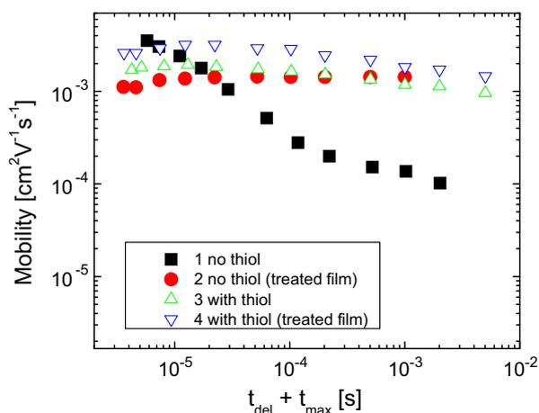
**Fig. 7.** Charge carrier mobility of 4 different RR-P3HT/PCBM bulk-heterojunction solar cells: as produced (filled squares), annealed (filled circles), thiol added (open up-pointing triangles), annealed film with thiol (open down-pointing triangles).
