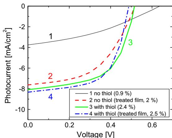
**Fig. 2.** Current–voltage ( $I$ – $V$ ) curves in the fourth quadrant of 4 different RR-P3HT/PCBM bulk-heterojunction solar cells under illumination with solar simulator ( $1000 \text{ W/m}^2$ ,  $1.5 \text{ AM}$ ): as produced (thin line), annealed (thick dashed line), thiol added (thick line), thiol added and annealed film (thick dash dot line).
