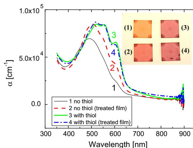
**Fig. 1.** Optical absorption coefficient of 4 different RR-P3HT/PCBM bulk-heterojunction solar cells: as produced (thin line), annealed (thick dashed line), thiol added (thick line), thiol added and annealed film (thick dash dot line).
