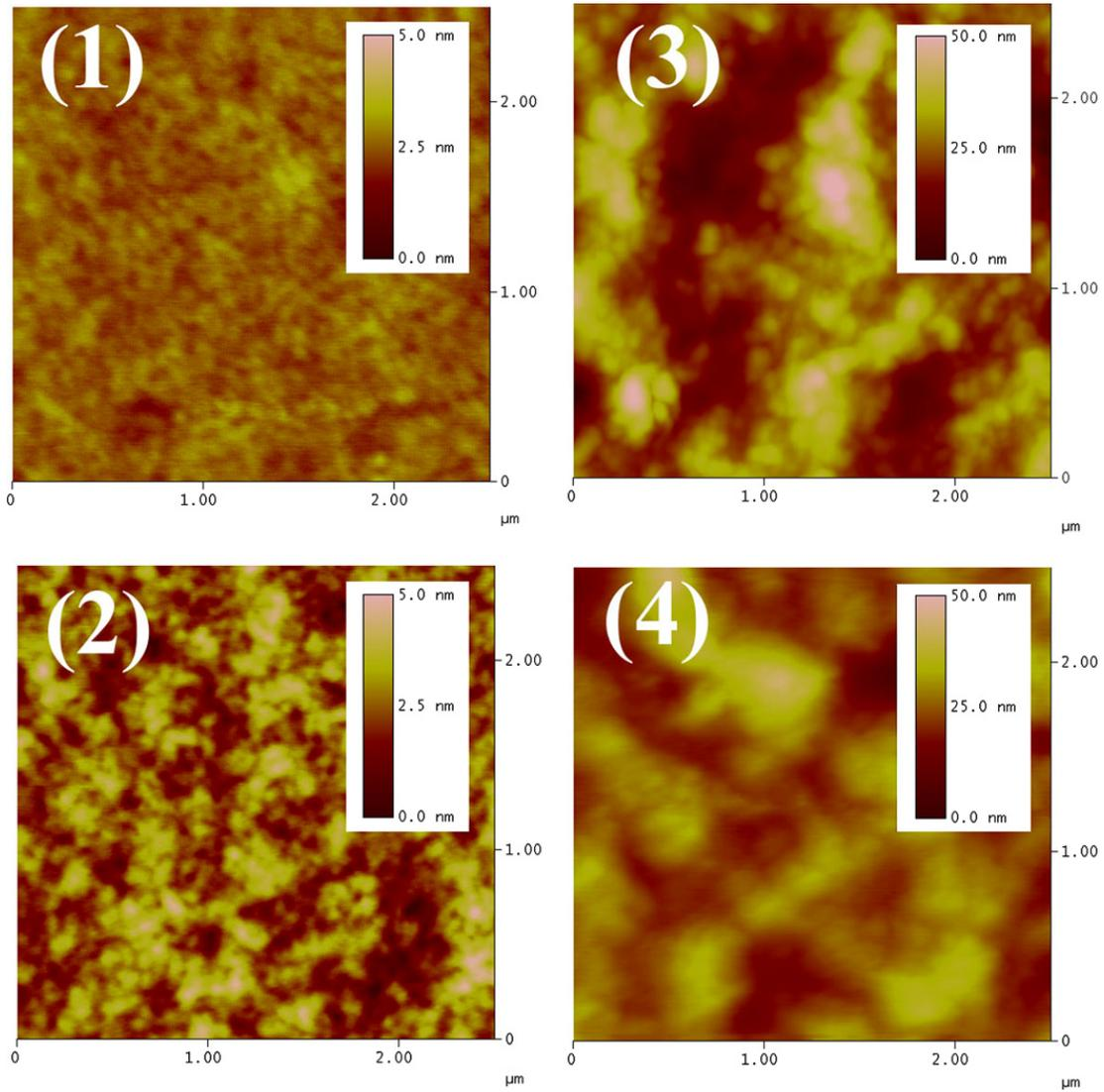
**Fig. 4.** Tapping mode AFM images of 4 different RR-P3HT/PCBM bulk-heterojunction solar cells: as produced (1), annealed (2), thiol added (3), thiol added and annealed film (4). The RMS surface roughness for all solar cells is 0.2 nm (cell 1), 0.6 nm (cell 2), 7.1 nm (cell 3), and 4.3 nm (cell 4).
