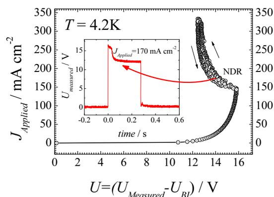
**Figure 4** Negative differential resistance regime at 4.2 K showing a reversible voltage breakdown. Inset: Voltage drop measured time-resolved in negative differential regime.
