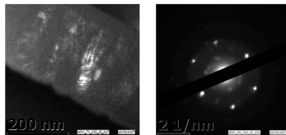
**Figure 3** (Right) Dark-field analysis of diode cross section shows similar orientation domains in growth direction. (Left) Diffraction pattern of  $C_{60}$  crystallite exhibits fcc hexagonal structure.
